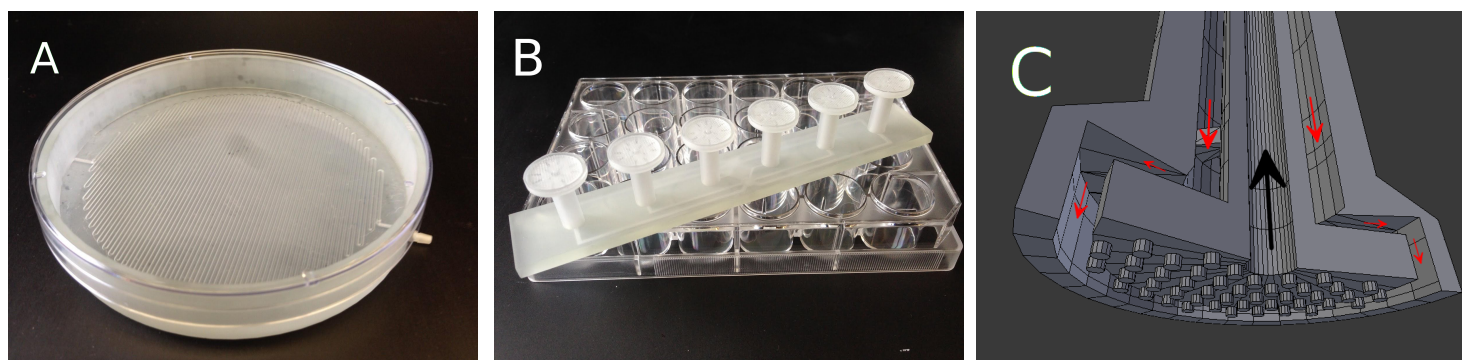
Figure 1: 3D printed devices. (A) 3" petri dish device. (B) 6 well prototype of 24 well plate insert. (C) Cross sectional CAD rendering of 'pipe in pipe' design. Red arrows indicate flow to the diffusion chamber and the black arrow is exhausted gas.
