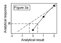
In this Figure, the solid line represents the true calibration function, while the broken line is the linear regression line. At a low concentration, which provides a response R, the fitted line provides a negative result.
