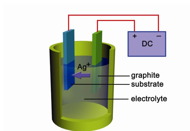
**Fig. S1.** Schematic set-up for the electrodeposition of Ag micro-hemispheres on ITO substrate.
