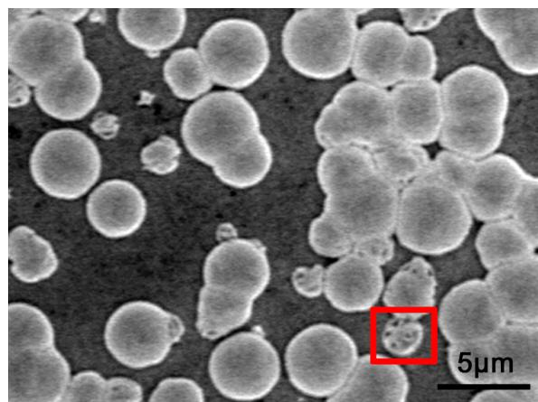
**Fig. S2.** SEM image of Ag micro-hemispheres with some imperfect ones (marked with red rectangular frame for attention).
