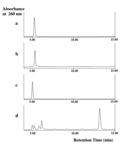
Reverse phase HPLC characterisation of products from the reaction of oligonucleotides **D** and **E** with ferrocene carboxylic acid N-succinimide ester (FNHS). Chromatograms for oligonucleotide **D** prior to (a) and after (b) incubation with FNHS and for oligonucleotide **E** prior to (c) and after (d) incubation with FNHS.
