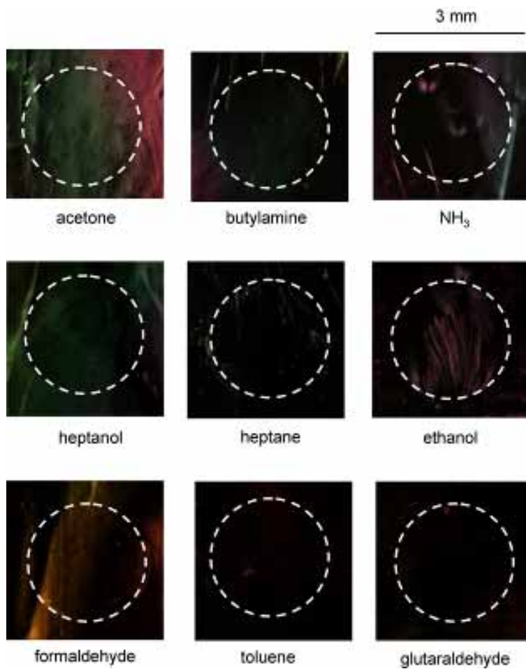
Fig. S1 Optical micrographs of a thin layer of liquid crystal 5CB ( \sim 6 \mu\text{m} ) sandwiched between a DMOAP - coated surface and an aminated surface patterned with circular domains of 1 mM of \text{Cu}^{2+} ions. Before 5CB was filled, the metal-decorated surface exposed different reagents.
