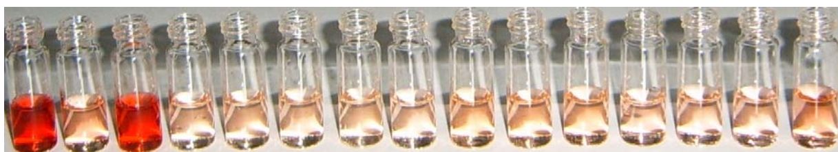
Figure S9. Different solutions of compound I and copper ions in water at pH 7.4 [20 mM HEPES, 135 mM NaCl] ( 1.0 \times 10^{-4} and 5.0 \times 10^{-5} mol/L, respectively) in the presence of anion ( 6.0 \times 10^{-5} mol/L). From left to right: no copper ions and no anion; no anion, \text{CN}^- , \text{SCN}^- , \text{F}^- , \text{ClO}_4^- , \text{HSO}_4^- , \text{Br}^- , \text{H}_2\text{PO}_4^- , \text{NO}_2^- , \text{SO}_4^{2-} , \text{I}^- , \text{Cl}^- , \text{IO}_3^- , the mixture.
