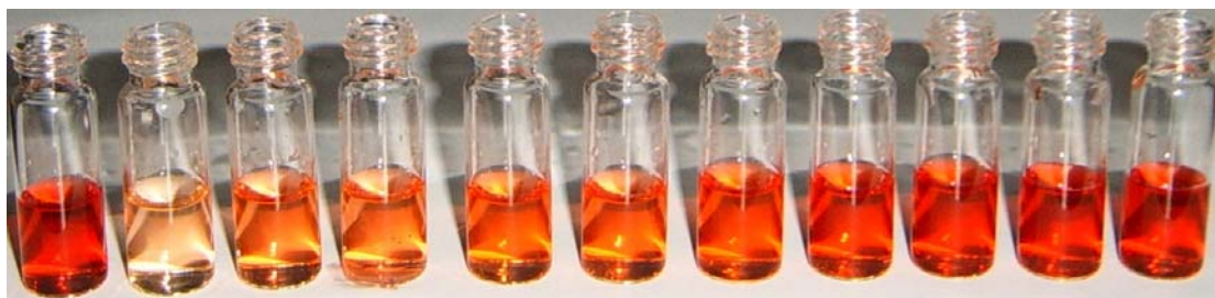
Figure S7. Different solutions of compound I and copper ions ( 1.0 \times 10^{-4} and 5.0 \times 10^{-5} mol/L, respectively) in water at pH 7.4 (20 mM HEPES, 135 mM NaCl) in the presence of different concentrations of \text{CN}^- . From left to right ( \times 10^{-5} mol/L): no copper ions and no cyanide, 0, 1.0, 2.0, 3.0, 4.0, 5.0, 6.0, 7.0, 8.0 and 9.0.
