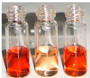
Figure S8. From left to right: compound I ( 1.0 \times 10^{-4} mol/L), compound I ( 1.0 \times 10^{-4} mol/L )+ \text{Cu}^{2+} ( 5.0 \times 10^{-5} mol/L), compound I ( 1.0 \times 10^{-4} mol/L )+ \text{Cu}^{2+} ( 5.0 \times 10^{-5} mol/L)+ \text{CN}^- ( 6.0 \times 10^{-5} mol/L) at pH 7.4 (20 mM HEPES, 135 mM NaCl).
