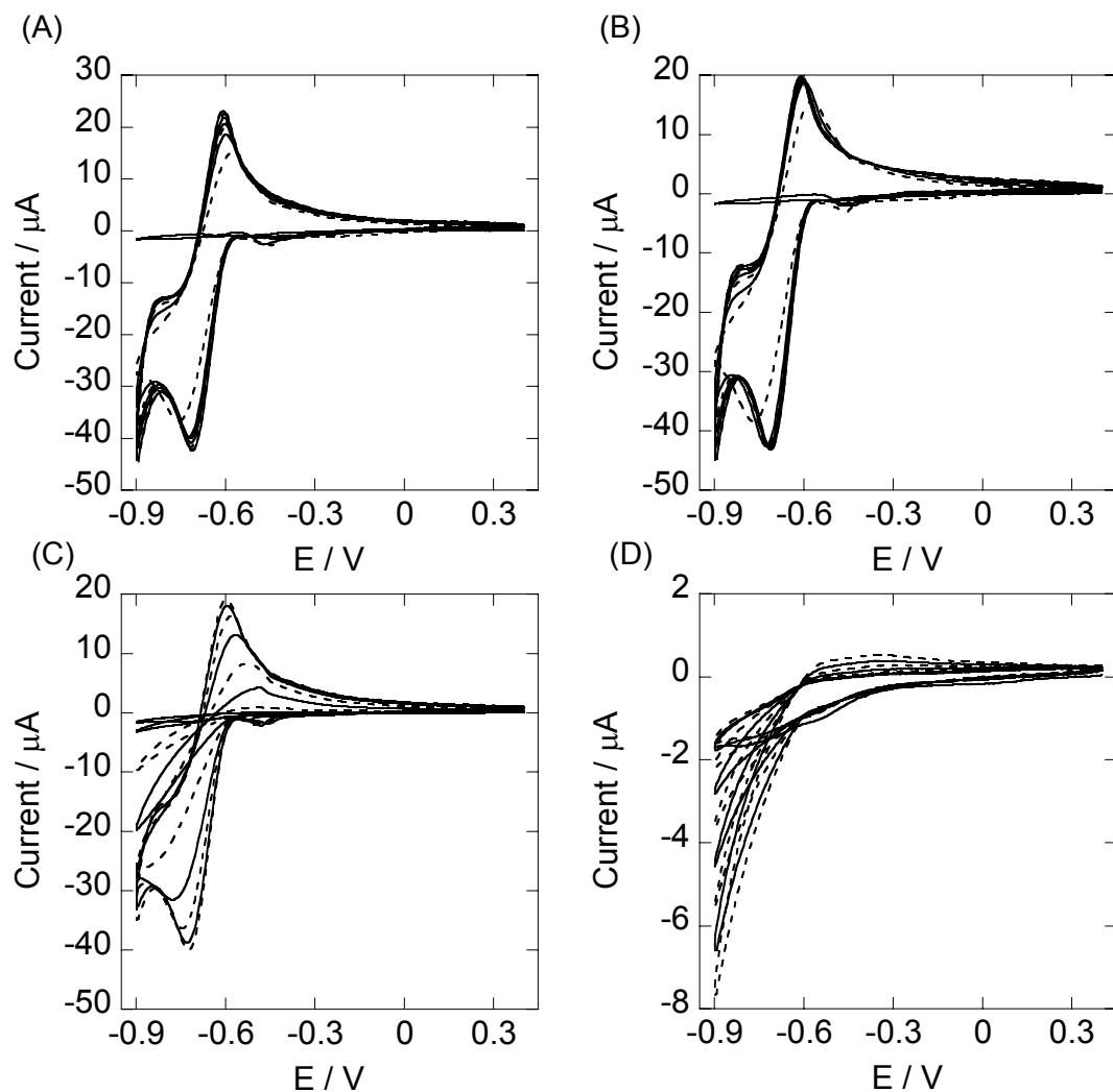
Figure S2. Cyclic voltammograms of a series of ten cycles on the glassy carbon electrode in 0.1 M phosphate buffer solution containing 0.5 mM cisplatin. DNA (from herring sperm) concentrations are (A) 30 ng/mL, (B) 300 ng/mL, (C) 3.0  $\mu$ g/mL and (D) 30  $\mu$ g/mL.
