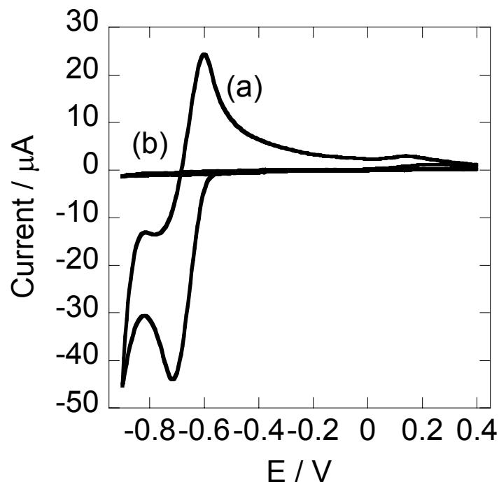
Figure S1. Cyclic voltammograms in the cisplatin-free buffer solution obtained (a) on the electrode, which had been used for the three times of potential scan in the 0.5 mM cisplatin solution and (b) after polishing the electrode surface.
