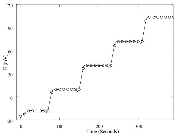
**Figure. S9** Time response curve of  $\text{Hg}^{2+}$  ion selective electrode E-1 based on **3**.
