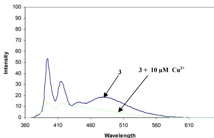
**Figure S2.** Fluorescence emission spectra of **3** (5  $\mu\text{M}$ ) in the presence of 10  $\mu\text{M}$  of  $\text{Cu}^{2+}$  ions in THF. Excitation wavelength was 343 nm.
