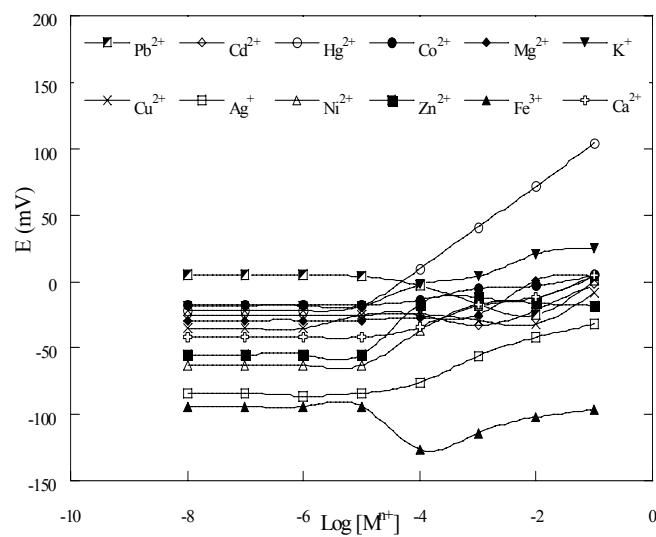
**Figure. S4.** Potentiometric response curves of ISEs based on **3** towards different metal ions.
