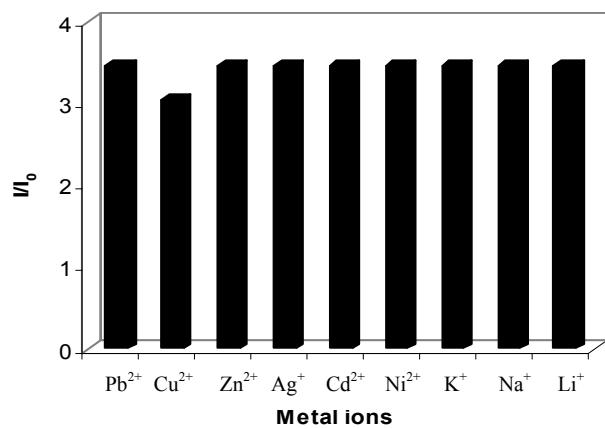
**Figure S3.** Fluorescence response of **3** (5  $\mu\text{M}$ ) on addition of 10  $\mu\text{M}$  of  $\text{Hg}^{2+}$  ions in the presence of 50  $\mu\text{M}$  of other selected metal ions .
