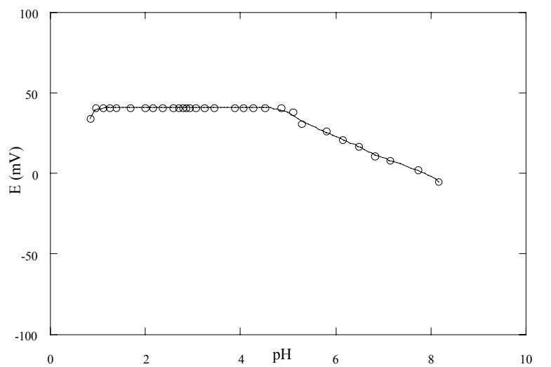
**Figure S5.** Effect of pH on potential response of  $\text{Hg}^{2+}$  ion selective electrode based on **3**.
