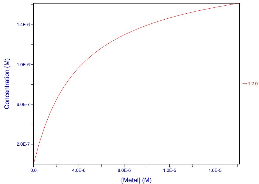
**Figure. S8** Concentration plot for 1:2 ( $\text{Hg}^{2+}$  : ligand) obtained from SPECFIT data.
