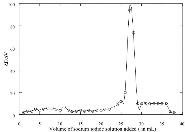
**Figure S6.** Derivative plot for titration of  $\text{Hg}^{2+}$  ions vs iodide ions using  $\text{Hg}^{2+}$  ion selective electrode E-1 as indicator electrode.
