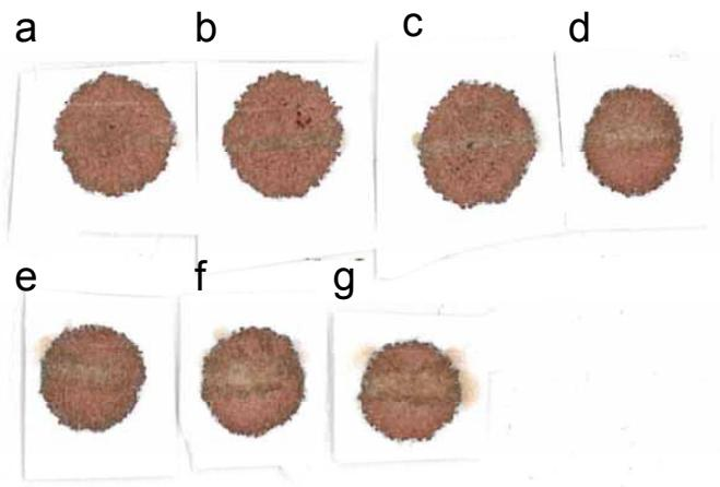
**Fig. S1** Photograph of DBS on Whatman 31 ETF after analysis by DESI-MS/MS at (a)  $3 \mu\text{L min}^{-1}$ , (b)  $5 \mu\text{L min}^{-1}$ , (c)  $10 \mu\text{L min}^{-1}$ , (d)  $15 \mu\text{L min}^{-1}$ , (e)  $20 \mu\text{L min}^{-1}$ , (f)  $25 \mu\text{L min}^{-1}$ , (g)  $30 \mu\text{L min}^{-1}$
