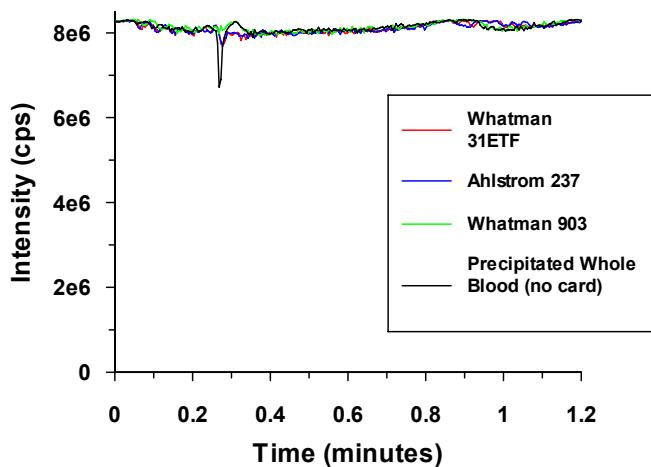
**Fig. S2** Post-column infusion (PCI) experiment detailing UPLC-MS/MS suppression of sitamaquine response after extraction from untreated (a) and treated specialty card types. Note the varying suppression intensity in solvent front using all papers, and secondary area of suppression using FTA paper. Proper analyte peak chromatographic conditions and retention time are essential to minimize suppression from card and ensure reproducible results.
