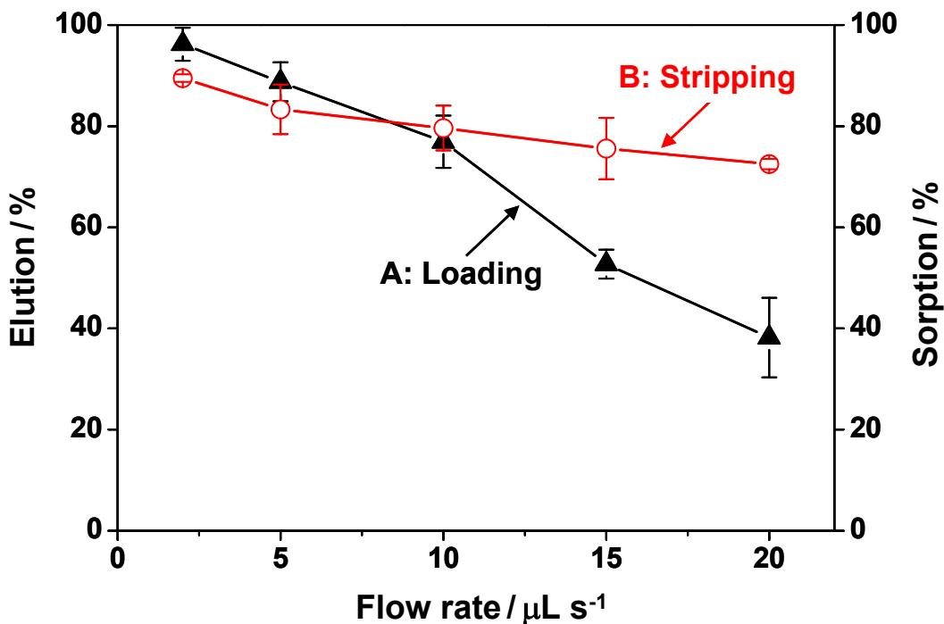
**Fig. S1.** (A) The dependence of adsorption efficiency of Se(VI) on the sampling flow rate and (B) the dependence of elution efficiency of the retained Se(VI) on the elution flow rate. Sample volume: 1000  $\mu\text{L}$ , 1.5  $\mu\text{g L}^{-1}$  Se(VI); Sample loading flow rate: 5.0  $\mu\text{g L}^{-1}$ ; Eluent (0.5 M  $\text{HNO}_3$ ): 50  $\mu\text{L}$ ; Elution flow rate: 5.0  $\mu\text{L s}^{-1}$ .
