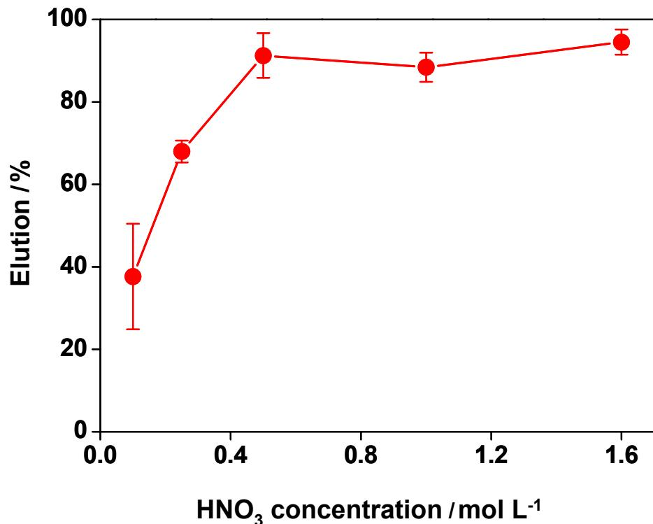
**Fig. S2.** The dependence of elution efficiency of Se(VI) on the concentration of eluent ( $\text{HNO}_3$ ).
