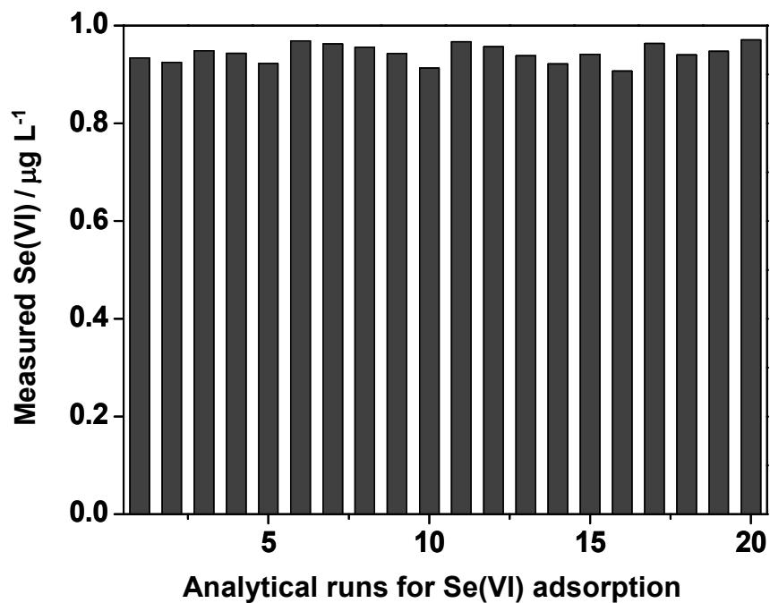
**Fig. S3.** The adsorption of Se(VI) in the presence of Se(IV) retention/Se(0) accumulation on the thio-ESM. Sample: a mixture of  $1.0 \mu\text{g L}^{-1}$  Se(IV) and  $1.0 \mu\text{g L}^{-1}$  Se(VI),  $1000 \mu\text{L}$ ; Sample loading flow rate:  $5.0 \mu\text{g L}^{-1}$ ; Eluent ( $0.5 \text{ mol L}^{-1}$   $\text{HNO}_3$ ):  $50 \mu\text{L}$ ; Elution flow rate:  $2.0 \mu\text{L s}^{-1}$ .
