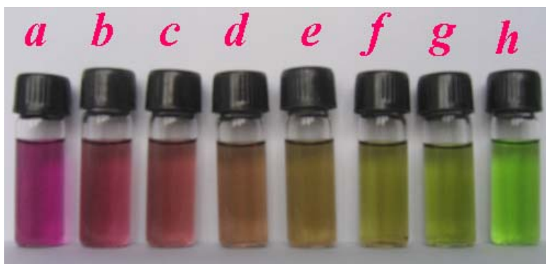
Fig. S8 Colour changes of TAR-Pd sensing solutions ( 1.0 \times 10^{-5} \text{ mol L}^{-1} in 80% (v/v) acetonitrile-water) titrated with increased amounts of \text{Me}_2\text{SnCl}_2 (a \rightarrow h: 0, 0.50 equiv., 1.00 equiv., 1.50 equiv., 2.00 equiv., 2.50 equiv., 3.00 equiv. and 4.00 equiv.).
