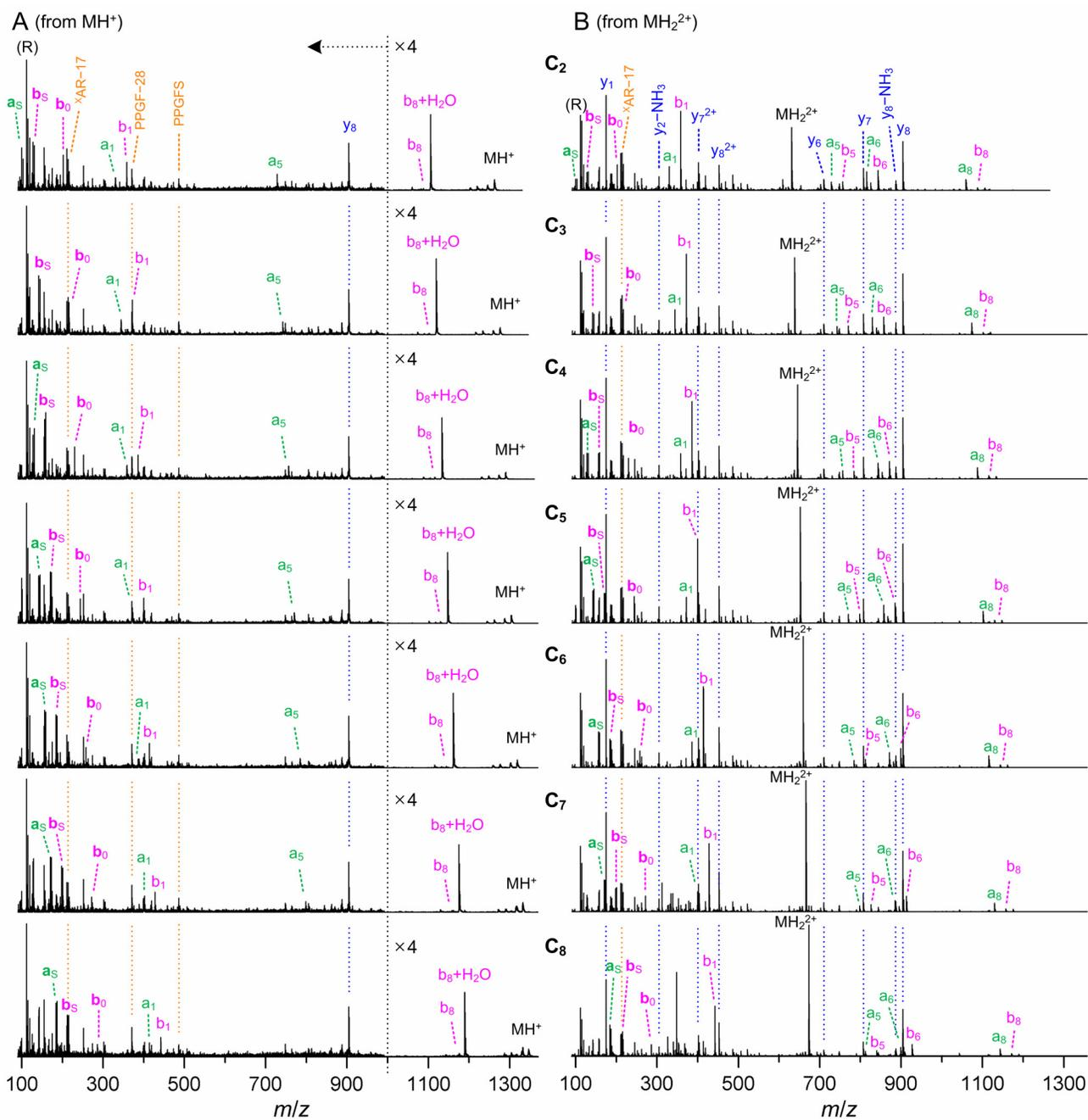
**Fig. S2** (A) MALDI-MS/MS spectra of singly-protonated MBIT-linked bradykinin (*N*-Ac-XA-RPPGFSPFR) obtained using TOF/TOF (Applied Biosystems 4700 Proteomics Analyzer, Foster City, CA) and (B) ESI-MS/MS spectra of doubly-protonated MBIT-linked bradykinin obtained using Q-TOF (Waters Q-TOF Premiere, Manchester, UK). The a, b, and y-type ions are colored in green, magenta, and blue, respectively.
