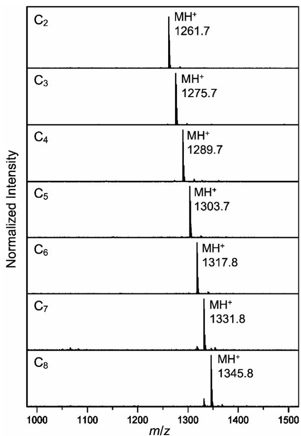
**Fig. S1** MALDI mass spectra of aliphatic (C<sub>2</sub>–C<sub>8</sub>) MBIT-linked bradykinin (*N*-Ac-**X**A-RPPGFSPFR).
