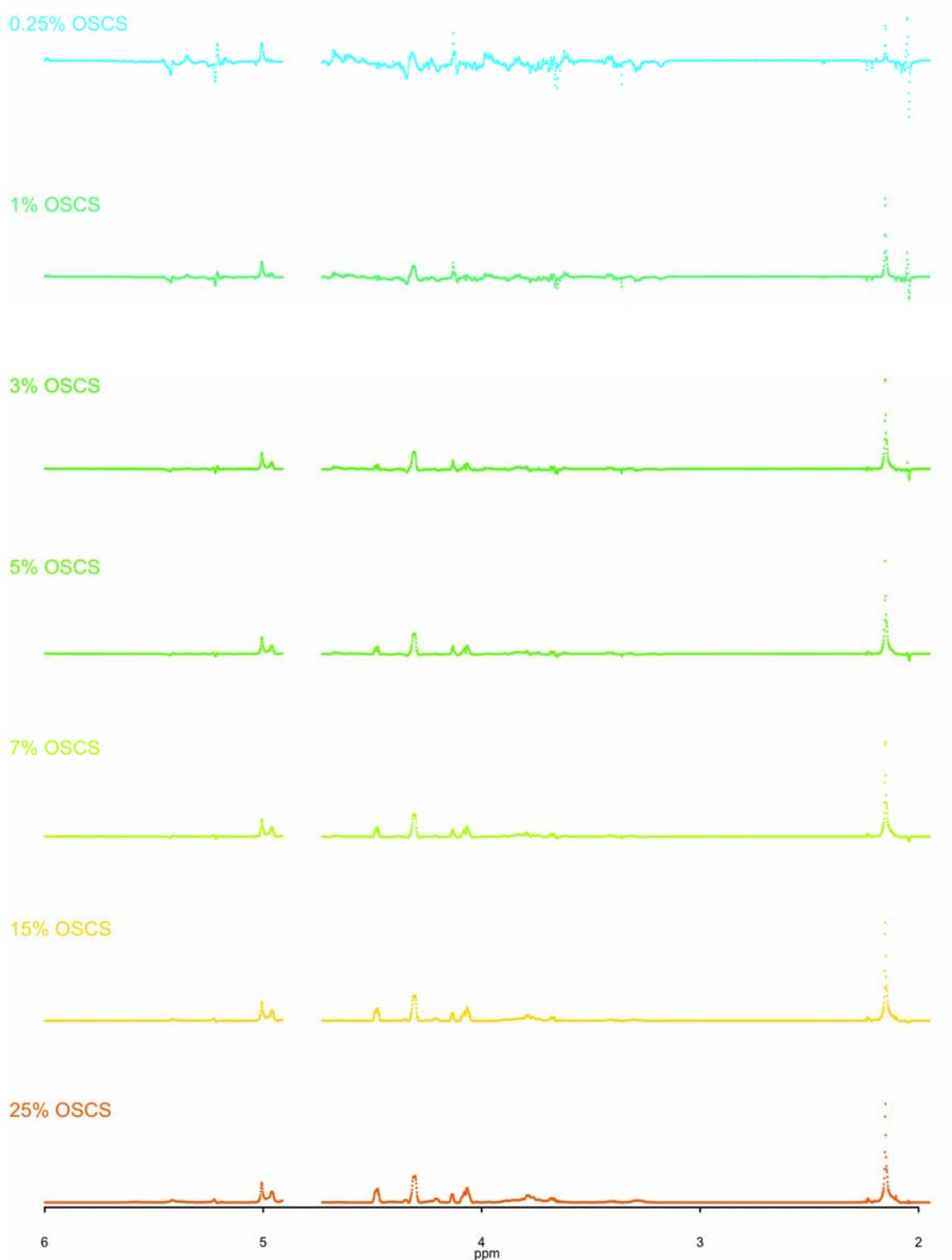
**Figure S2.** Reconstructed spectra of the OSCS [0.25 - 25 %] contaminant. The above spectra were created by subtracting the heparin 2D-COS power spectrum away from the specific OSCS [0.25 -25 %] plus heparin dataset power spectrum. The power spectrum is the diagonal of the 2D-COS spectrum, or the variance of the covariance matrix.
