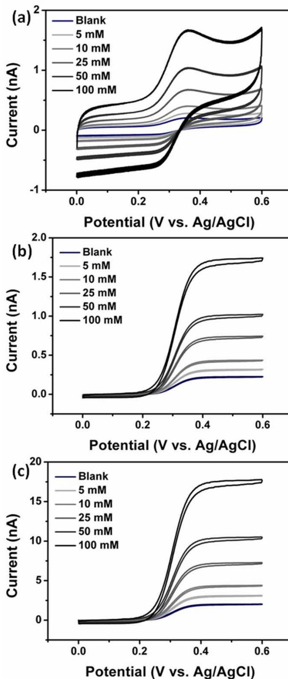
**Fig S3:** Optimisation of Electrolyte conditions: cyclic voltammograms of increasing concentrations of glucose at a single nanowire electrode, at  $50 \text{ mV s}^{-1}$  in the presence of (a) 1 mM FcCOOH,  $1 \text{ mg ml}^{-1}$  GOx in 100 mM PBS, pH 7.0, (b) 1 mM FcCOOH,  $1 \text{ mg ml}^{-1}$  GOx in 10 mM PBS, pH 7.4, and (c) 10 mM FcCOOH,  $1 \text{ mg ml}^{-1}$  GOx in 10 mM PBS, pH 7.4.
