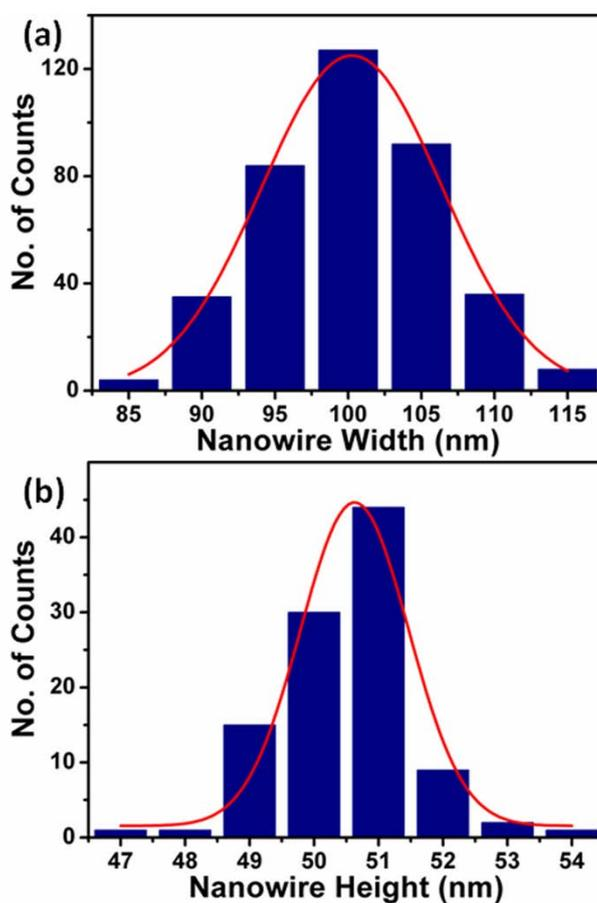
**Fig S1:** Histograms showing the distribution of widths (a) and heights (b) of nanowires electrodes fabricated by EBL, obtained from SEM and AFM analysis, respectively. Solid red lines are Gaussian fits to the data.
