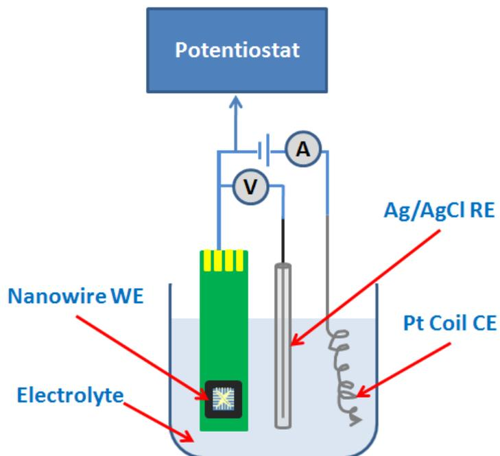
**Fig S2:** Schematic representation of three-electrode electrochemical cell setup employed. PCB mounted nanowire electrodes served as working electrodes (WE), coupled with a platinum coil counter electrode (CE) and Ag/AgCl KCl Sat., reference electrode (RE).
