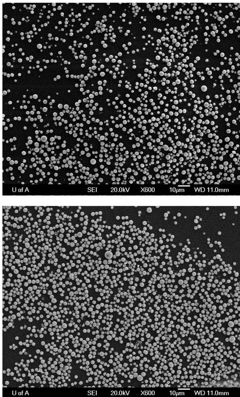
**Supplementary Fig. 1:** An overview of carbon clad zirconia particles (top), two times sulfonated carbon clad zirconia particles (bottom). Different batches do not differ in morphology in carbon or sulfur content. No breakage or change in morphology can be seen for particles which go through 2 x sulfonation (2 hour stirring) and a stringent washing procedure with various solvents and 1% wt/wt NaOH.
