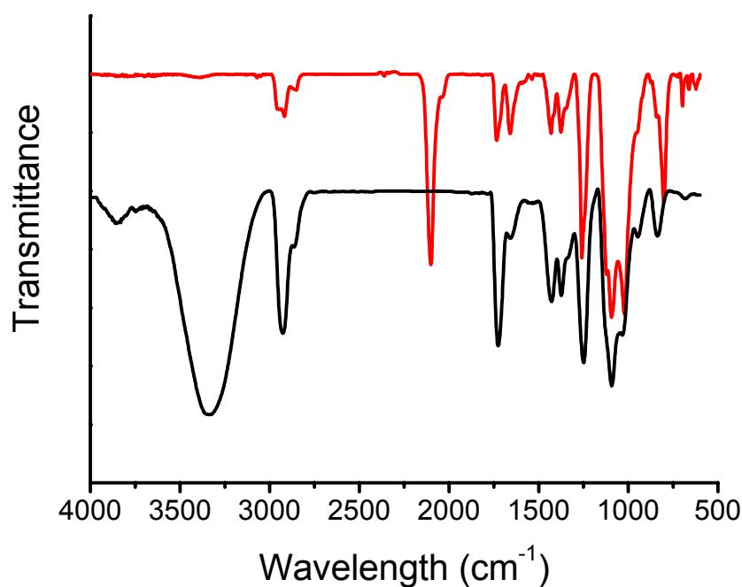
**Fig. S8** FTIR spectra. Black curve: PVA film; red curve: PVA film with azide functionality.
