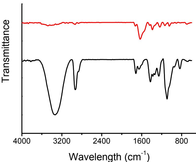
**Fig. S7** FTIR spectra. Black curve: PVA film chemosensor; red curve: PVA film containing DNS and EDTA.
