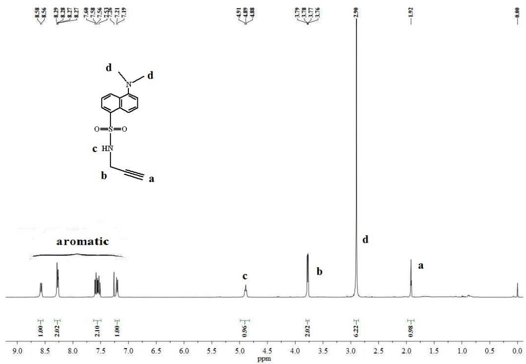
**Fig. S4** <sup>1</sup>H NMR spectrum of DNS-propyne (in CDCl<sub>3</sub>).
