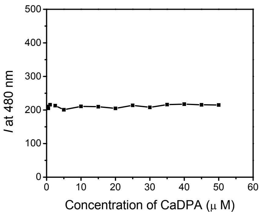
**Fig. S2** Fluorescence intensity of DNS (Intensity at 480 nm, reference dye) on the PVA film chemosensor as the concentration of CaDPA was varied. ( $\lambda_{\text{ex}} = 270 \text{ nm}$ )
