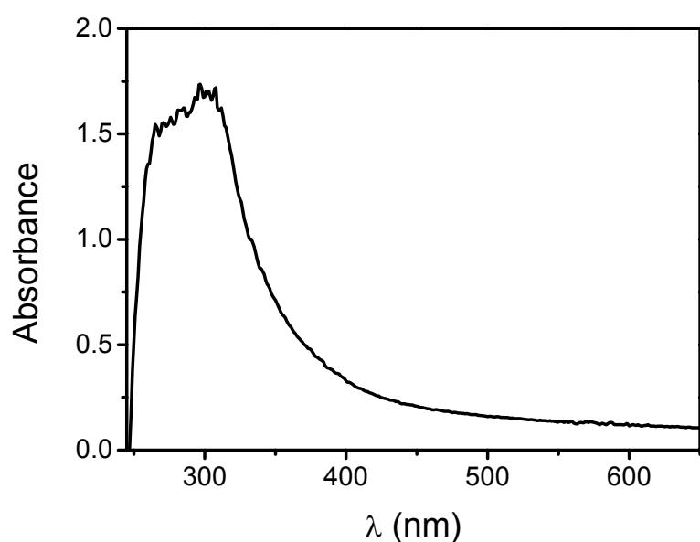
**Fig. S1** Absorption spectrum of the PVA film chemosensor.
