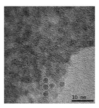
**Fig. S1** Bright field TEM image of 0.5 h refluxed TLA–ZnS QDs. Some clusters are encircled.
