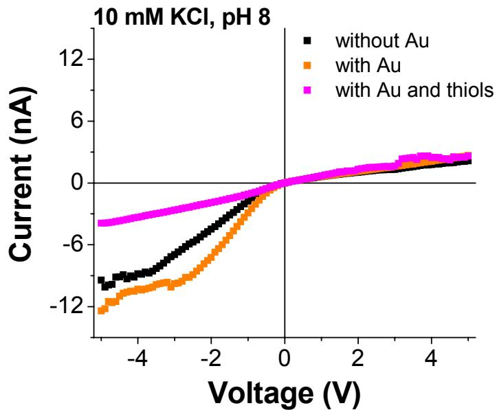
**Figure S2.** Ion current through a single nanopore before and after depositing a 22.5 nm thick gold layer, followed by chemisorption of hydrophobic thiols C18. The recordings were performed in 0.1 M KCl pH 8.
