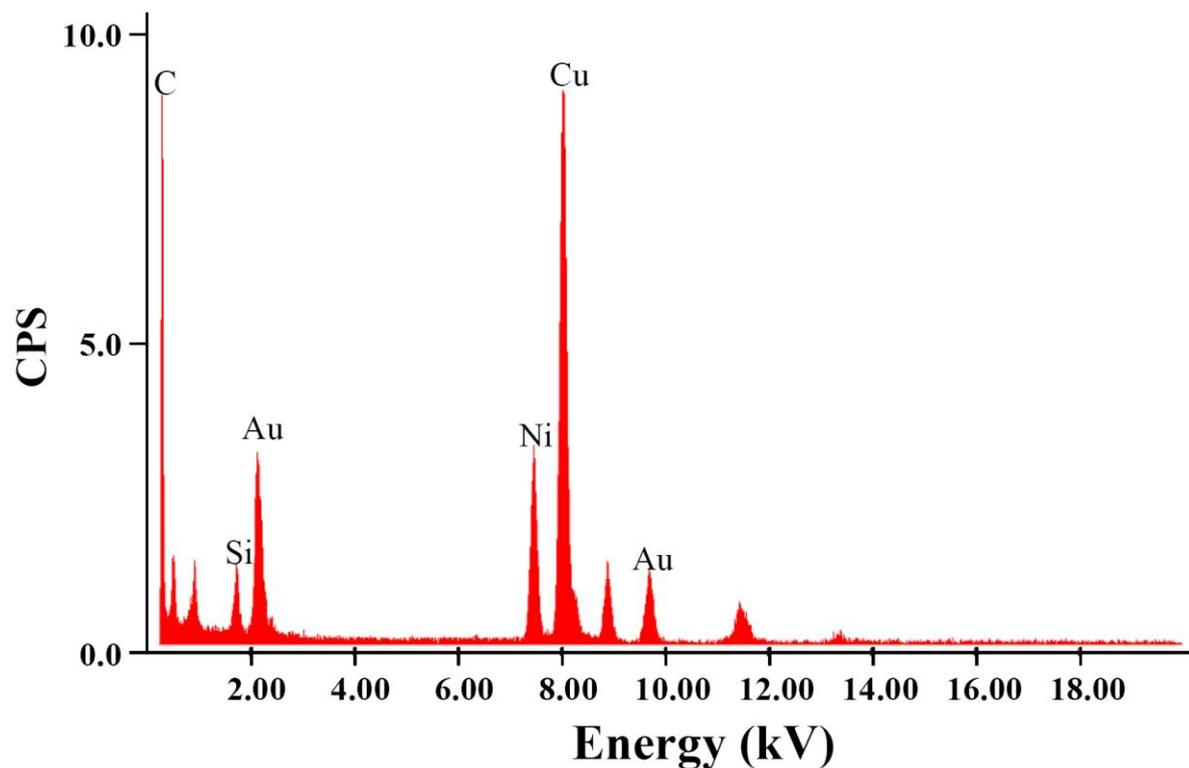
**Fig. S3** EDS spectrum of the Au NPs indicating the presence of Cu atoms on the NPs. After Au NPs reacted with  $\text{Cu}^{2+}$ ,  $\text{Pb}^{2+}$ , and 2-ME, the particles were purified and dipped on a carbon-coated nickel grid, and then dried at room temperature. Other conditions were the same as those described in Figure S2.
