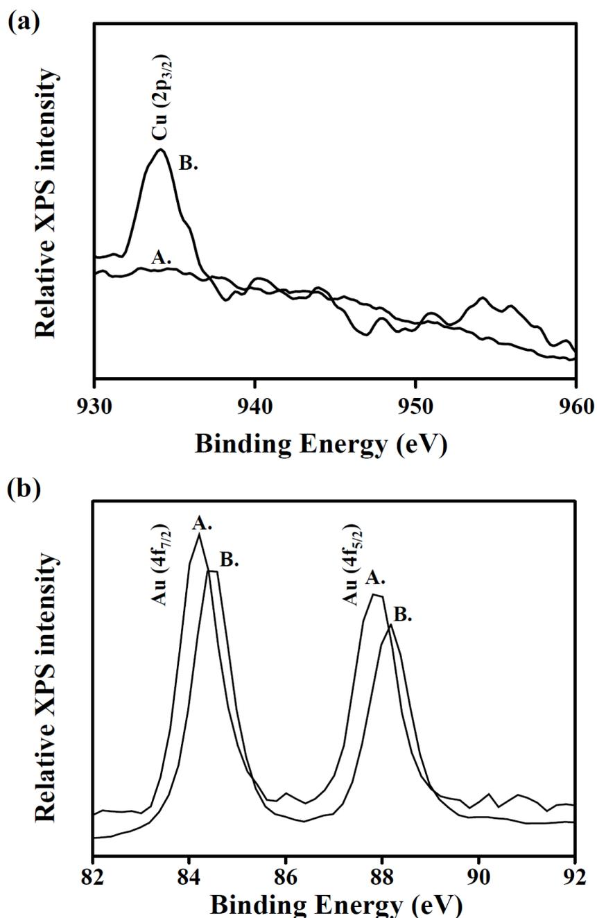
**Fig. S2** (a) Cu (2p<sub>3/2</sub>) and (b) Au (4f) core-level photoelectron spectra of BSA-Au NPs in the (A) absence and (B) presence of Cu<sup>2+</sup> (10 μM), 2-ME (1.0 M), and Pb<sup>2+</sup> (50 μM) in 5 mM glycine–NaOH solution (pH 12.0). The sample dosed onto silicon substrates and measured at room temperature. Other conditions were the same as those described in Figure 1.
