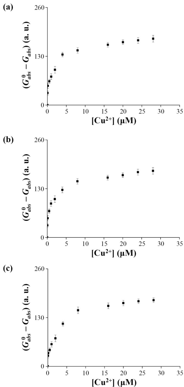
**Fig. S4** Analyses of representative (a) stream water, (b) sea water, and (c) tap water samples using the  $Pb^{2+}/2$ -ME-BSA-Au NPs/NCM probes. Diluted water samples (2.5-fold) were spiked with  $Cu^{2+}$  ions (0–30  $\mu M$ ). Other conditions were the same as those described in Figure 5.
