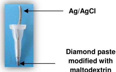
Fig. 1 Stochastic sensor based on maltodextrin.
