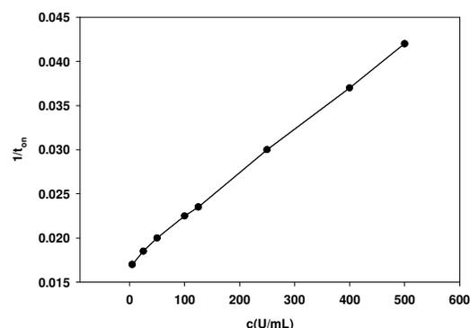
**Fig. 2** Calibration graph of maltodextrin based stochastic sensor.
