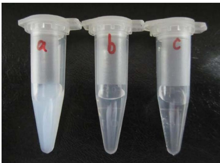
**Fig. S3** Photograph of dialyzed solution of (a) ionized PAA-AgNO<sub>3</sub> and (b) non-ionized PAA-AgNO<sub>3</sub> in the presence of 0.05 M NaCl, (c) the solution of 0.05 M NaCl.
