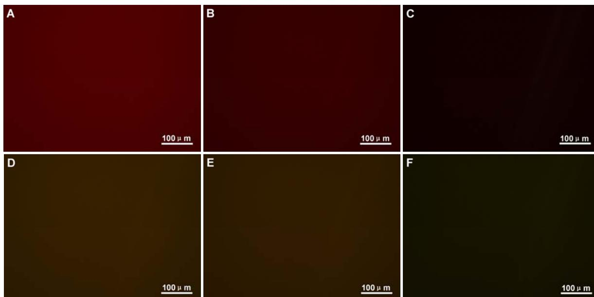
**Fig. S4** Fluorescence images of the as-prepared AgNCs solution (A, D) in the absence of  $\text{Cu}^{2+}$ , and in the presence of (B, E)  $10^{-4}$  M  $\text{Cu}^{2+}$ , and (C, F)  $10^{-3}$  M  $\text{Cu}^{2+}$ . Note: (A-C) under green light excitation and (D-F) under blue light excitation.
