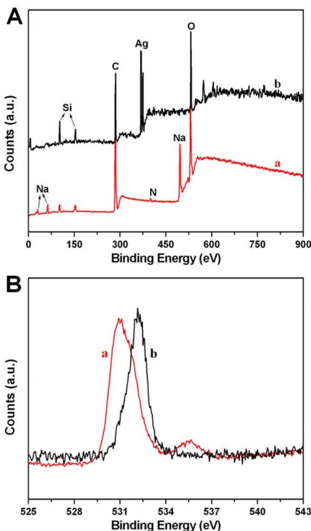
**Fig. S1** (A) XPS survey spectra of (a) the synthesized MPAA and (b) the suspension produced in the presence of high concentration of  $\text{Ag}^+$ ; (B) high resolution XPS for the O 1s signals: (a) MPAA and (b) the suspension.
