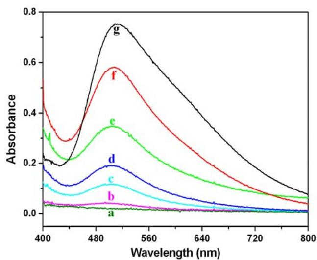
**Fig. S2** UV-vis spectra of MPAA-Ag<sup>+</sup> solution after different time of irradiation: (a) 0, (b) 120, (c) 150, (d) 160, (e) 170, (f) 180, (g) 190 s.
