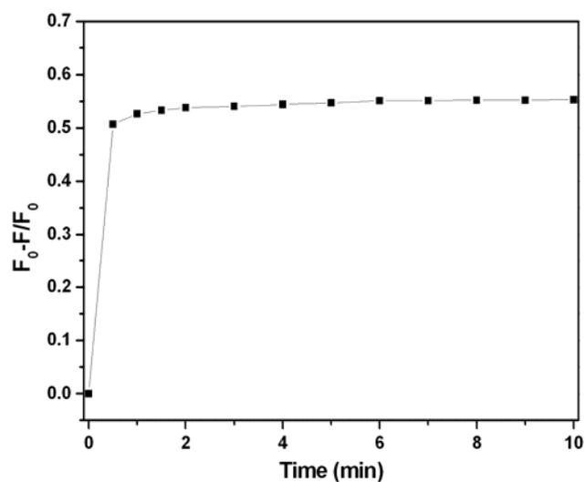
**Fig. S5** Plot of  $F_0 - F / F_0$  against time in the presence of  $2.5 \times 10^{-4}$  M  $\text{Cu}^{2+}$ .
