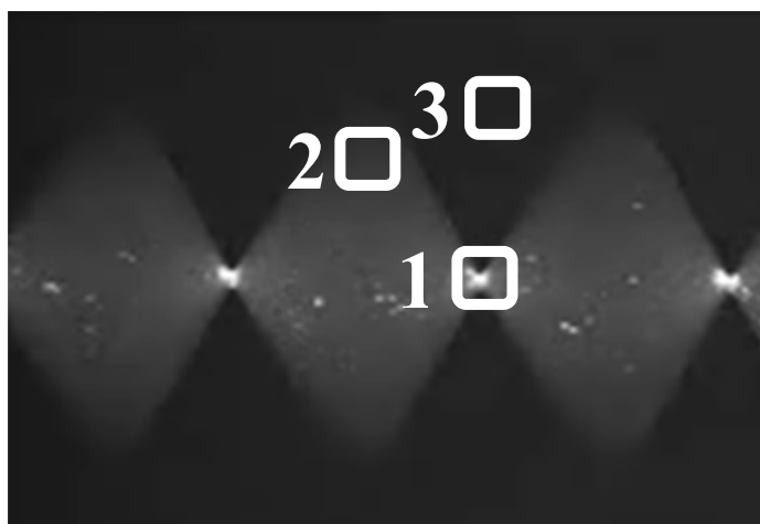
Fig. ESI-1: Regions of interest (ROIs) indicated as described in the text. Three different areas were selected to determine the enrichment of fibril concentration in the capture zone using the fluorescence intensities in each region. The areas depicted here are larger than the actual ROIs used for ease of viewing.
