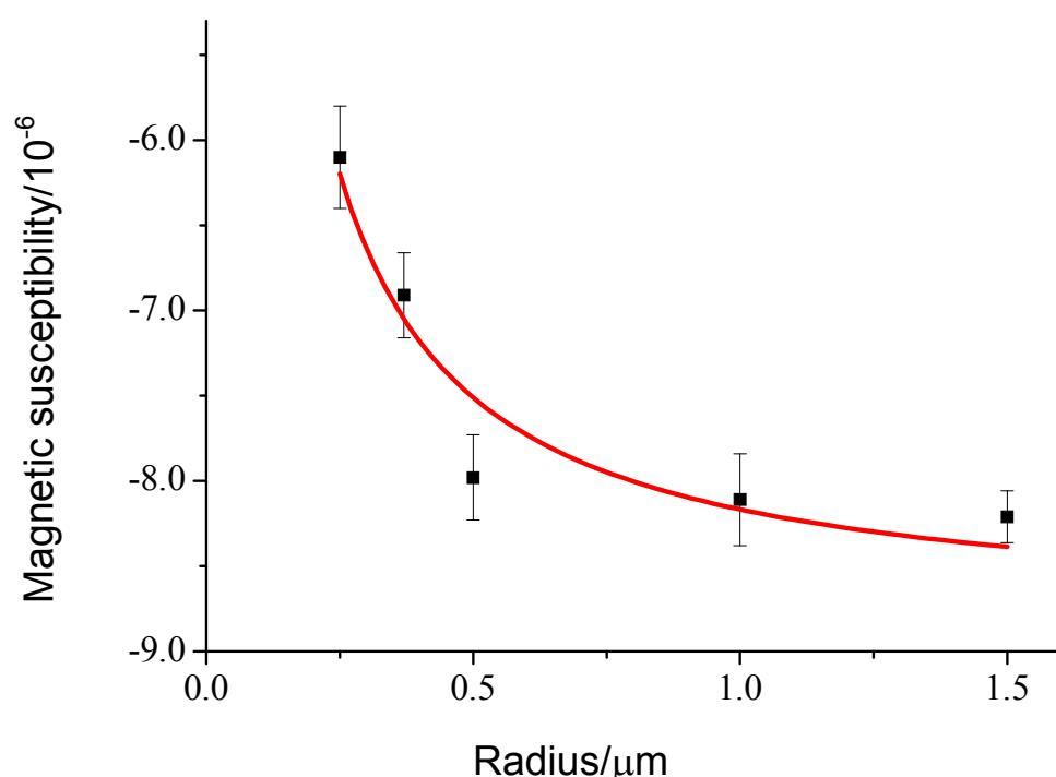
**Fig. SF-3** Relationship between the magnetic susceptibility determined from the velocity and the radius for the polystyrene particles determined by the Brownian motion method. The plots were fitted with the equation (4) and the two parameters were obtained as the bulk magnetic susceptibility,  $\chi_b = -(8.82 \pm 0.27) \times 10^{-6}$ , and the interfacial magnetic susceptibility,  $\chi_i = (0.21 \pm 0.03) \times 10^{-12} \text{ m}^{-1}$ .
