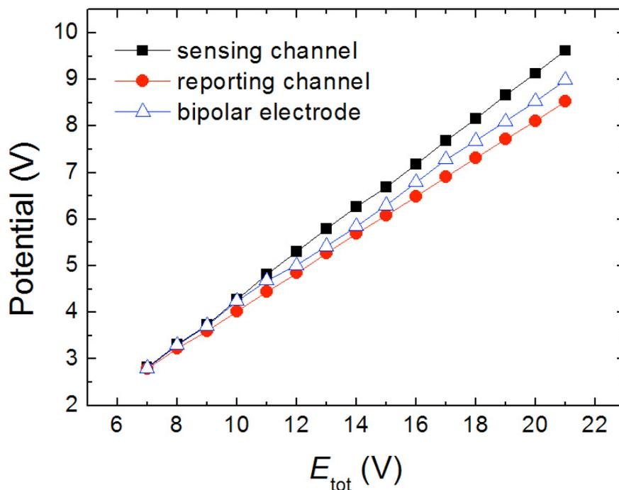
**Figure S1.** Potential profiles of microbands in the sensing (■) and the reporting channels (●), and the bipolar electrode (△) constructed by connecting the two separate microbands.
