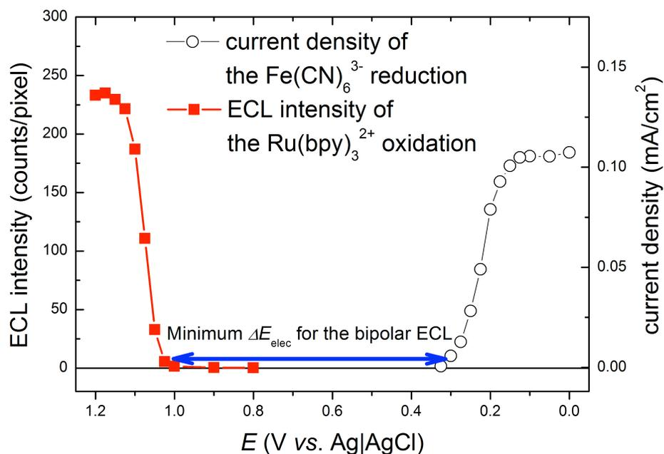
**Figure S3.** Plot of ECL intensity and current density as a function of electrochemical potential. The plots were obtained from separate experiments. The minimum  $\Delta E_{\text{elec}}$  required for the ECL reporting is estimated to be 0.67 V based on the difference between the onset potentials for ECL and the reduction of  $\text{Fe}(\text{CN})_6^{3-}$ .
