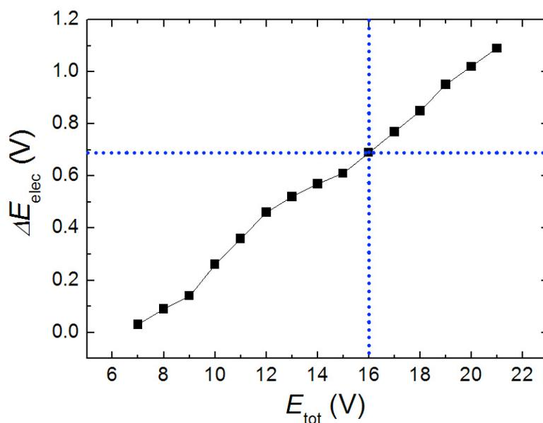
**Figure S2.** Plot of the potential difference ( $\Delta E_{\text{elec}}$ ) between cathodic and anodic poles of the BPE, calculated from the potential profiles plotted in Figure S1, as a function of the driving voltage ( $E_{\text{tot}}$ ). ECL was observed with a minimum driving potential of  $E_{\text{tot}} = 16.0$  V, which is equivalent to  $\Delta E = 0.69$  V (shown as blue dotted lines).
