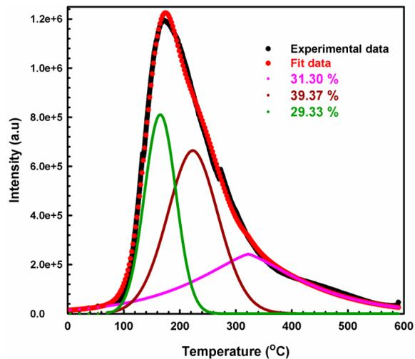
**Figure S3** NH<sub>3</sub>-TPD spectra and a deconvolution of each peak of hexagonal aluminosilica monoliths fabricated with a Si/Al mole ratio of 4. To determine the amount and strength of acid sites of the mesoporous aluminosilica particles quantitatively, we deconvoluted the peaks around 100 °C to 500 °C using a Gaussian function with temperature as the variant.
