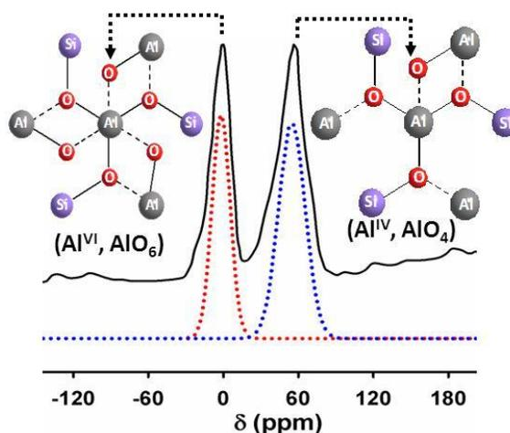
**Figure S1** <sup>27</sup>Al MAS NMR spectra and a deconvolution of each peak of aluminosilica carriers fabricated with a Si/Al ratio of 4.
