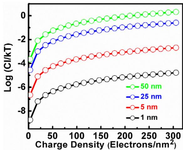
**Figure S-1.** The plots of  $\text{Log}(CI/kT)$  versus charge density for nanorods with radii of 1, 5, 25, and 50 nm.
