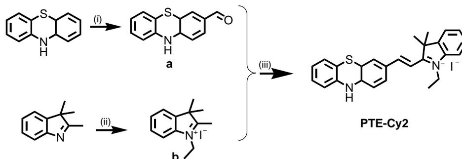
**Scheme S1.** Synthetic route of dye **PTZ-Cy2**. i) DMF, 1,2-dichloroethane, POCl<sub>3</sub>, reflux 8 h, yield 63%; ii) toluene, CH<sub>3</sub>CH<sub>2</sub>I, reflux 10 h, yield 92%; iii) ethanol, piperidine, reflux 12 h, yield 65%.
