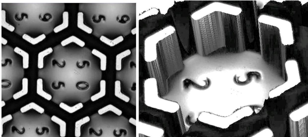
**Fig. S1.** 2D image and 3D rendition of the split wall microcup. The 2D image was acquired using an Olympus LEXT 3D Measuring Laser Microscope OLS-4000 and converted to a 3D rendition (50° altitude from the horizontal) with accompanying software.
