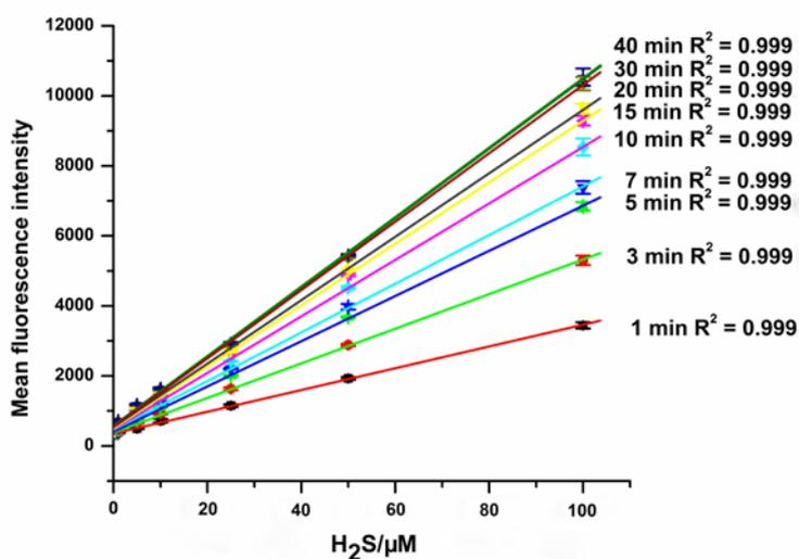
Figure S6. The relationship of mean fluorescence intensity and H<sub>2</sub>S concentrations for C-6Az (100 μM). The concentrations of H<sub>2</sub>S are 0 μM, 100 μM, 1 mM, 10 mM and 100 mM respectively and the fluorescence intensity of each sample was recorded at 1 h, 3 h, 5 h, 7 h, 10 h at 37 °C, pH=7.4, Ex/Em = 340 /445 nm (filter: 420 nm, PMT: medium) through top-reading using Molecular Devices FlexStation III microplate reader.
