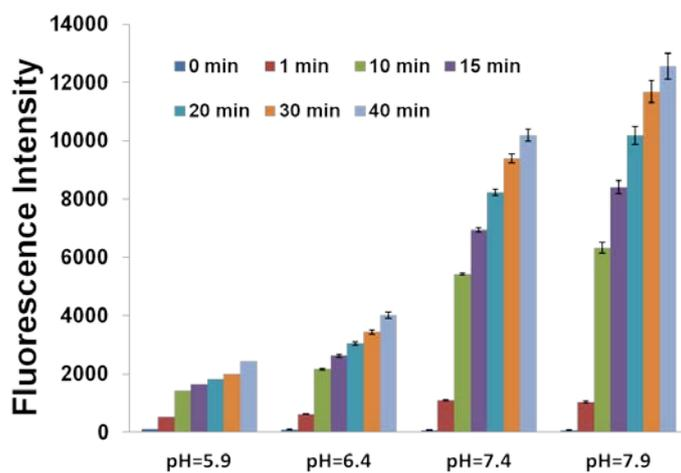
Figure S8. Photostability of C-7Az degassed PBS solution with UV light irradiation and the addition of NaHS (the last black column). The Sample was irradiated at 1, 3, 5, 7, 10, 15, 20, 30 min (365 nm, 11 mW/cm<sup>2</sup>) and the fluorescence emission was measured at 37 °C, Ex/Em = 340 /445 nm (filter: 420 nm, PMT: medium) through top-reading using Molecular Devices FlexStation III microplate reader. The last column is the same solution with the addition of 100 μM C-7Az.
