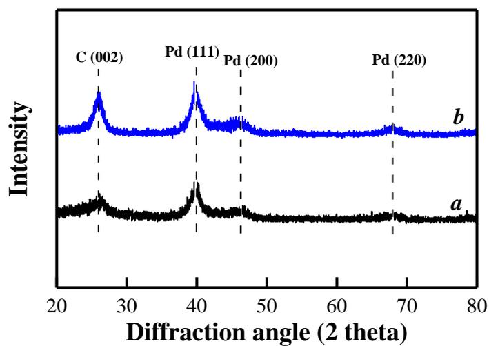
Fig. S11. XRD patterns of the graphene/Pd (curve *a*) and CNT/Pd (curve *b*) samples.
