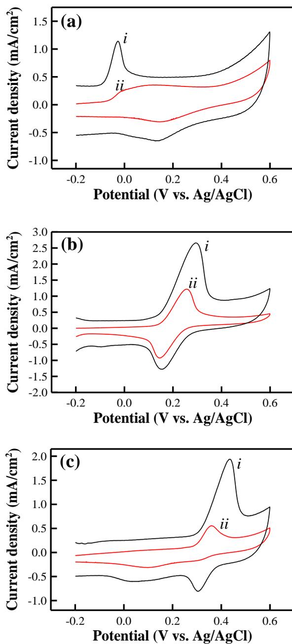
Fig. S12. Cyclic voltammograms of IL/graphene/Pd (curves *i*), and IL/CNT/Pd (curves *ii*) electrodes recorded in (a) 1 mM AA, (b) 1 mM DA, and (c) 1 mM UA PBS solution at a potential scan rate of 50 mV/s. A hydrophilic 1-ethyl-3-methylimidazolium–tetrafluoroborate IL is this case.
