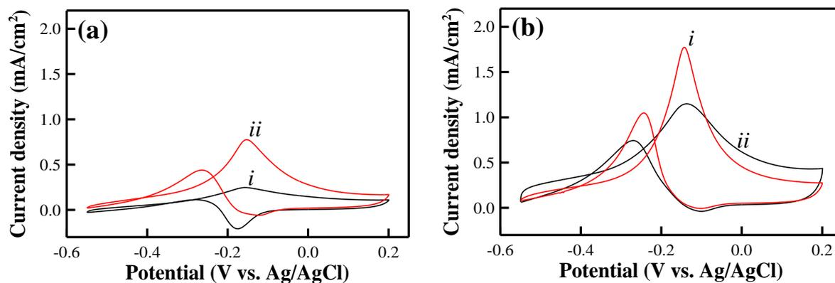
Fig. SI4. Cyclic voltammograms of the graphene/Pd (curves *i*) and CNT/Pd (curves *ii*) electrodes recorded in 5 mM glucose NaOH solution at a potential scan rate of 10 mV/s. The electrodes are (a) without and (b) with BMI-PF<sub>6</sub> IL incorporation, respectively.
