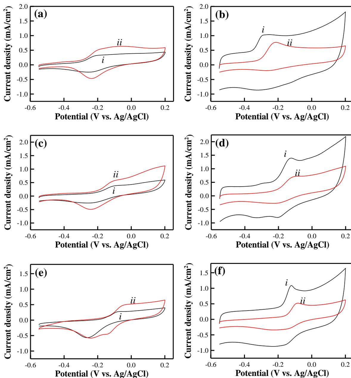
Fig. SI3. Cyclic voltammograms of the graphene/Pd (curves *i*) and CNT/Pd (curves *ii*) electrodes recorded at a potential scan rate of 50 mV/s in NaOH solution that contains 1 mM AA ((a), (b)), 1 mM DA ((c), (d)), and 1 mM UA ((e), (f)). The electrodes are without ((a), (c), (e)) and with ((b), (d), (f)) BMI-PF<sub>6</sub> IL incorporation.
