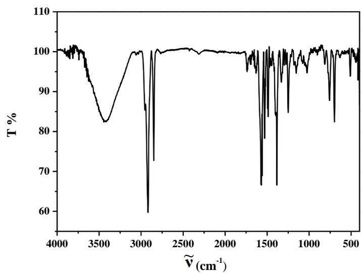
**Figure S26.** IR spectrum of  $(\text{TPAQCOOH})_2\text{Irpic}$
