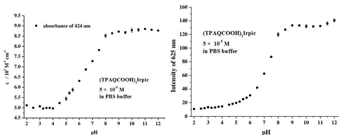
**Figure S14.** pH-Dependent changes in molar absorption coefficients (424 nm) and emission intensity (625 nm) of the probe  $(\text{TPAQCOOH})_2\text{Irpc}$  in aqueous PBS buffers and the corresponding error bars were provided.
