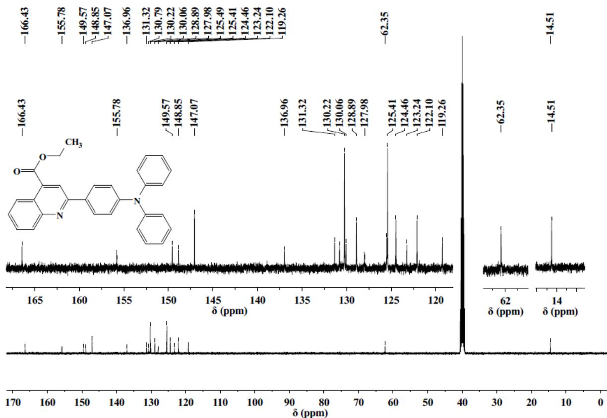
Figure S18.  $^{13}\text{C}$  NMR of TPAQCE in  $\text{DMSO-}d_6$
