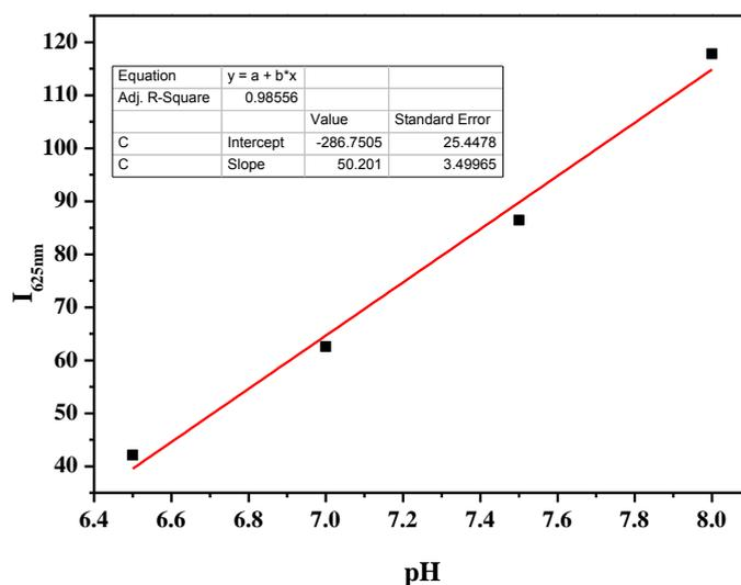
**Figure S13.** A plot of emission intensity of  $(\text{TPAQCOOH})_2\text{Irpc}$  at  $I_{625\text{nm}}$  vs pH (6.50 – 8.00) in aqueous buffer solutions. The red solid curve is fitting line of experimental data with relative coefficient  $R = 0.985$ .
