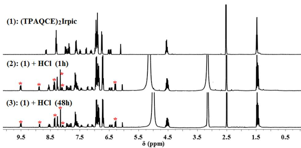
**Figure S6.** Aromatic part of the <sup>1</sup>H NMR in DMSO-*d*<sub>6</sub>: (TPAQCE)<sub>2</sub>Irpic (1); addition of ca. 20-30 equiv of HCl (ca. 2-3% in methanol / DMSO-*d*<sub>6</sub>) to the (TPAQCE)<sub>2</sub>Irpic solution for 2h (2); addition of ca. 20-30 equiv of HCl (ca. 2-3% in methanol / DMSO-*d*<sub>6</sub>) to the (TPAQCE)<sub>2</sub>Irpic solution for 48h (3). The six new peaks appeared by addition HCl to the solution of (TPAQCE)<sub>2</sub>Irpic are marked with \*.
