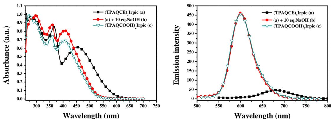
**Figure S1.** UV-vis absorption (normalized) and emission (excited at 400nm) spectra of: (a, ■), DMSO solution of (TPAQCE)<sub>2</sub>Irpc; (b, ●), solution (a) in presence of 10 equiv of aqueous NaOH; (c, ▽), DMSO solution of (TPAQCOOH)<sub>2</sub>Irpc.
