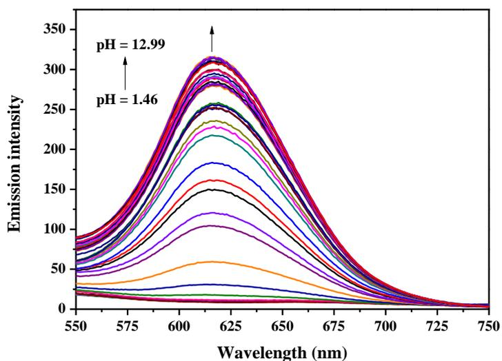
**Figure 16.** pH-Dependence of the emission spectra of  $(\text{TPAQCOOH})_2\text{Irpic}$  in ethanol: $\text{H}_2\text{O} = 3:7$  (containing 0.1 M NaCl) at concentration of  $5.0 \times 10^{-5}$  M.
