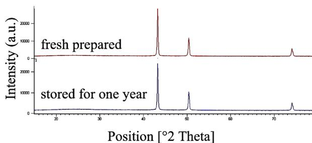
**Figure S2.** XRD patterns of fresh fabricated Cu@C-A NWs and the same samples stored for one year..
