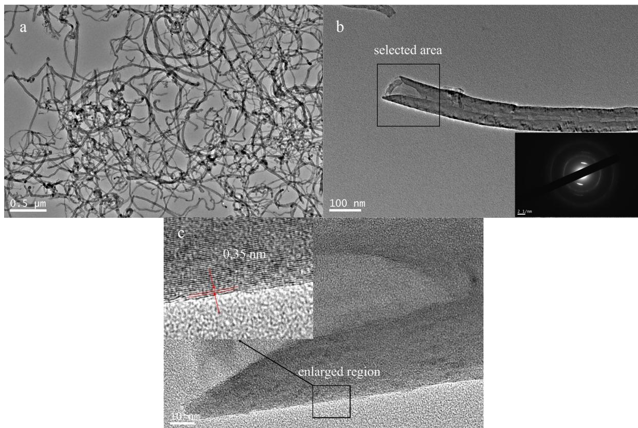
**Figure S5.** a) Low magnification TEM image of MWCNTs, b) TEM image of an individual MWCNT and inset is corresponding SAED pattern. c) High-resolution TEM image showing the multilayer sidewalls of a MWCNT and top left inset is enlarged region from edge area.
