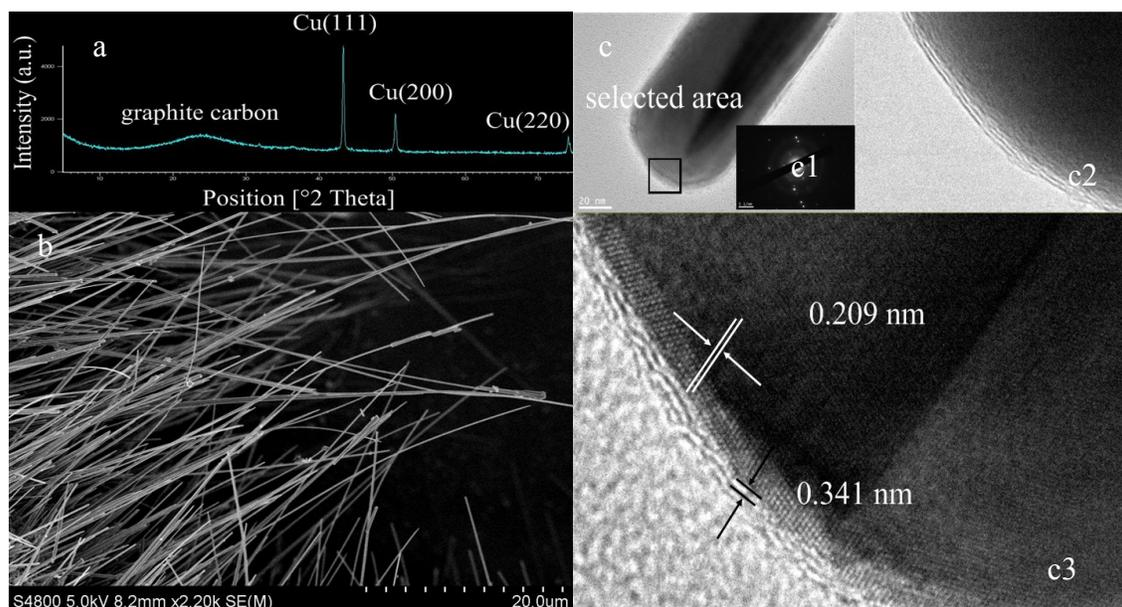
**Figure S4.** a) XRD-pattern of the as-obtained fresh products after dried in the atmosphere of nitrogen. b) SEM image with low magnification of the final products fabricated by MOCVD method. c) HRTEM characterizations of a single Cu@C NW: c1) TEM image of core-shell NW and its corresponding SAED pattern, taken along the [110] zone axis perpendicular to the long axis of the nanowire. c2) Copper/graphite carbon interface on the surface of Cu NW core, c3) HRTEM image of selected area from c1.
