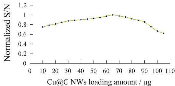
**Figure S8.** The signal-to-noise ratio (S/N) of the Nafion/Cu@C NWs/GCE in 50 mM NaOH to the injection of 50 μM glucose with increasing loading amount of Cu@C NWs.
