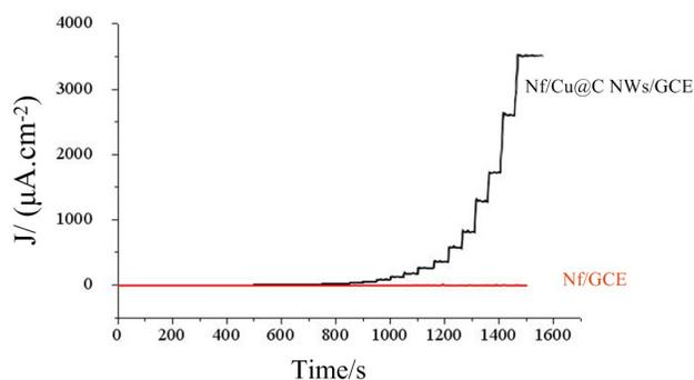
**Figure S11.** Amperometric responses of Nf/Cu@C NWs/GCE compared with blank Nf/GCE at 0.65 V to successive additions of glucose from 50 nM to 1 mM (double injections per concentration) in 50 mM NaOH.
