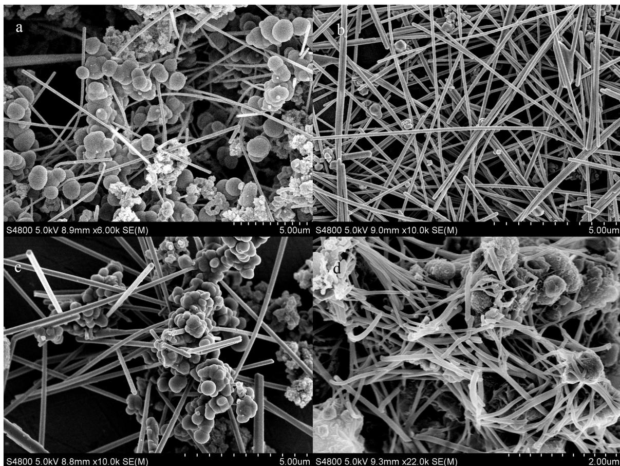
**Figure S9.** SEM images of Cu@C nanowires synthesized at different temperatures: (a) 140°C, (b) 150°C, (c) 160°C and (d) 170°C.
