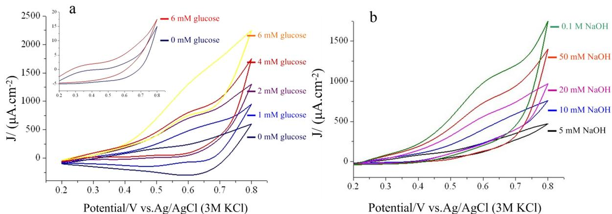
**Figure S7.** a) CVs of the Nf/Cu@C-A NWs/GCE and blank Nf/GCE (inset) in the presence of different concentrations of glucose from 0 to 6 mM, the electrolyte is 50 mM NaOH and the scan rate is 50 mV/s. b) Cyclic voltammograms of the Nafion/Cu@C NWs/GCE in different concentrations of NaOH from 5 mM to 0.1 M with 2 mM glucose concentration at a scan rate of 50 mV/s.
