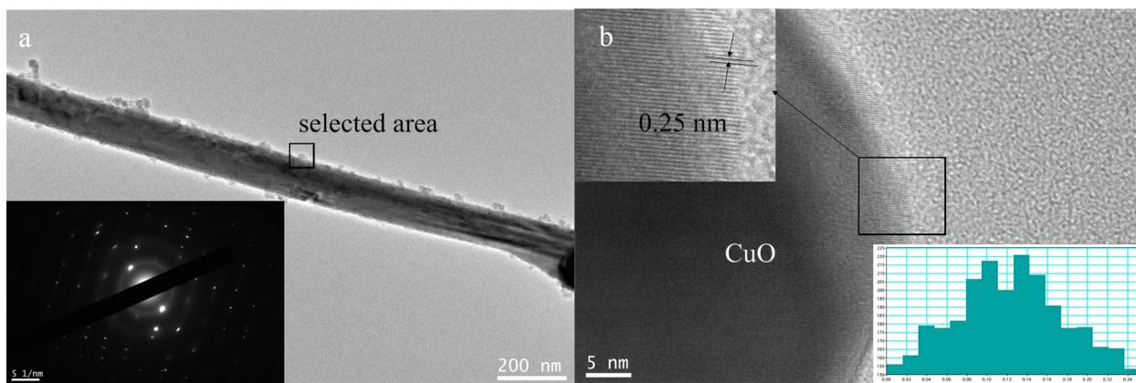
**Figure S13.** a) TEM images of as-prepared pure Cu NW sampled for glucose detection stored at ambient conditions over two months, and inset is corresponding SAED pattern. b) HRTEM image of a copper nanowire, the local enlarged image from the boxed region is also shown in this image, showing the lattice spacing of 0.25 nm corresponds to a d spacing of [110] crystal planes.
