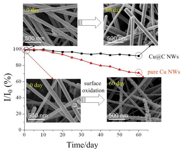
**Figure S14.** Long-term stability of the pure Cu NWs and Cu@C NWs modified sensors stored at ambient conditions over two months in 50 mM NaOH with addition of 1 mM glucose at 0.65 V.
