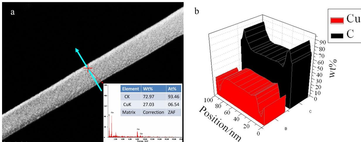
**Figure S3.** a) EDX spectra of selected area and b) Cu and C-distribution across the axis of a Cu@C nanowire synthesized via hydrothermal process by EDX-analysis.
