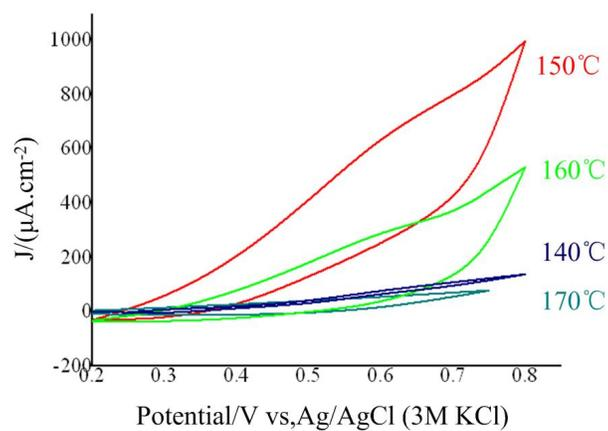
**Figure S10.** CVs of final products prepared under various temperature conditions modified electrodes with 2 mM glucose in 20 mM NaOH at scanrate of 50 mV/s.
