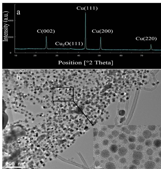
**Figure S6.** a) XRD pattern of as-prepared nanocomposites. b) Typical TEM micrographs of Cu@C-A NPs and their general size situation.
