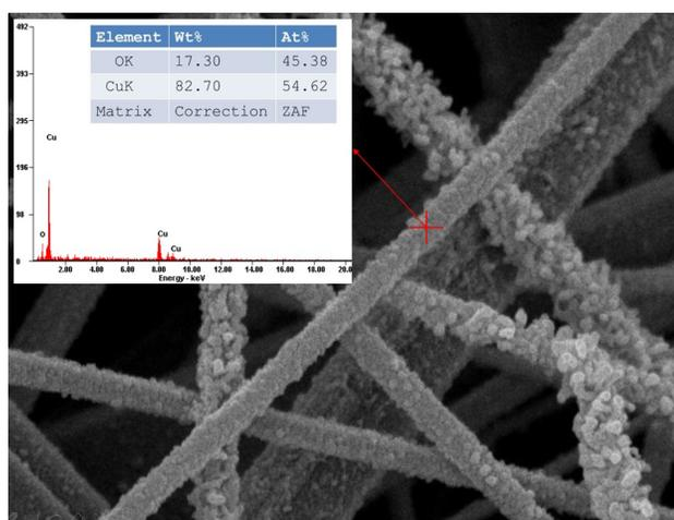
**Figure S15.** A typical SEM image and EDX spectrum of the CuO NWs stored in damp environment.
