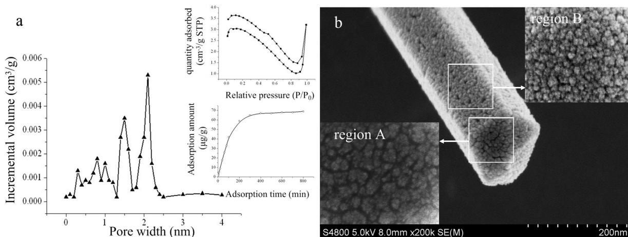
**Figure S12.** a) Nanopore size distributions within amorphous carbon shells coated on Cu NWs, top right inset shows nitrogen adsorption/desorption isotherms and bottom right inset is effect of adsorption time on glucose adsorption on Cu@C-A NWs. b) Partial enlarged view of a single Cu@C-A NWs which reveals surface of NW is rich in irregular voids and cracks.
