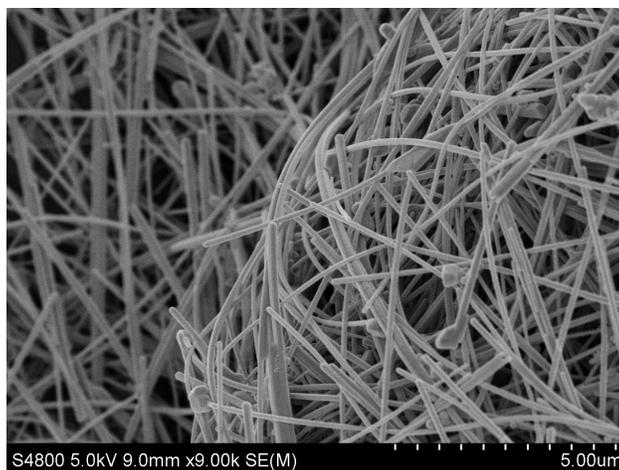
**Figure S1.** SEM image of as-prepared Cu@C NWs after centrifugation at a rotation speed of 4500 rpm.
