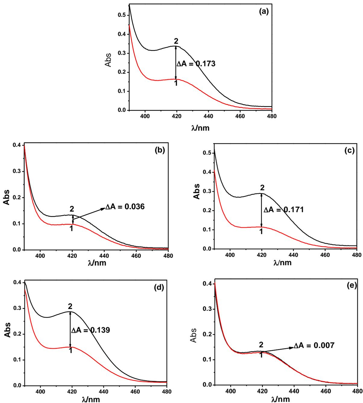
Fig. S7. UV-Vis absorption spectra of the peroxidation product ( $\text{ABTS}^{\bullet+}$ ) at 5 min of the  $\text{ABTS-H}_2\text{O}_2$  reaction in Tris- $\text{ClO}_4$  buffer ( $\text{pH} = 7.4$ ) containing  $0.1 \mu\text{M}$  hemin,  $140 \text{ mM Na}^+$  and  $0.1 \mu\text{M}$  (a) hairpin DNA 2; (b) hairpin DNA 3; (c) hairpin DNA 4; (d) hairpin DNA 5; (e) hairpin DNA 6: (1) adding  $10 \mu\text{M Pb}^{2+}$ , (2) adding  $10 \text{ mM K}^+$  to (1).
