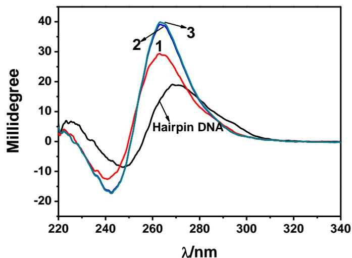
Fig. S3. CD spectra of 4  $\mu\text{M}$  hairpin DNA 1 in 20 mM Tris-ClO<sub>4</sub> buffer (pH = 7.4): (1) adding + 140 mM  $\text{Na}^+$  for 2 h; (2) adding 10 mM  $\text{K}^+$  to (1) for 2 h; (3) adding 10  $\mu\text{M}$   $\text{Pb}^{2+}$  to (1) for 2h, then adding 10 mM  $\text{K}^+$  for 2h.
