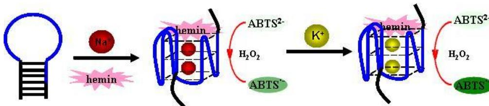
Fig. S2. Schematic of DNA conformational switches and the formed G-quadruplex DNAzyme functions
