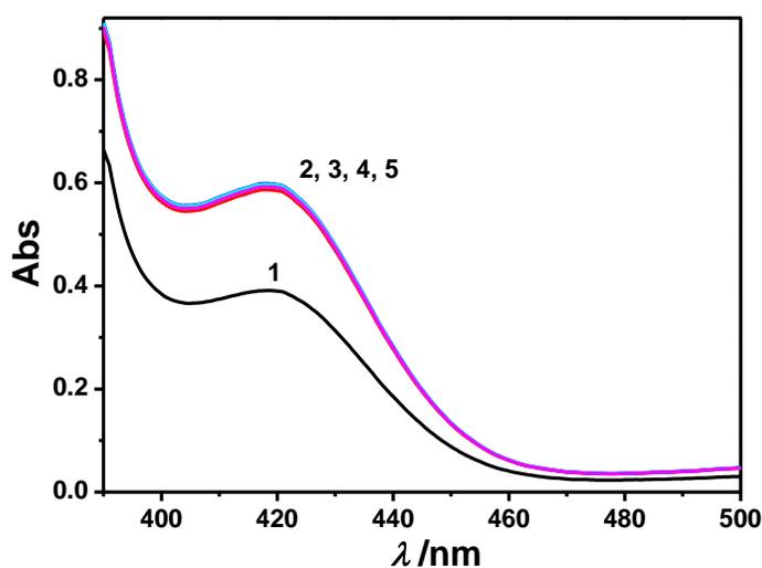
Fig. S5. UV-Vis absorption spectra of the peroxidation product (ABTS<sup>•-</sup>) at 5 min of the ABTS-H<sub>2</sub>O<sub>2</sub> reaction in Tris-ClO<sub>4</sub> buffer (pH = 7.4) containing 0.1  $\mu\text{M}$  hemin: (1) 0.1  $\mu\text{M}$  hairpin DNA 1 + 140 mM Na<sup>+</sup>; (2) 10 mM K<sup>+</sup> + (1); (3) 100 nM Pb<sup>2+</sup> + (2); (4) 1  $\mu\text{M}$  Pb<sup>2+</sup> + (2); (5) 10  $\mu\text{M}$  Pb<sup>2+</sup> + (2).
