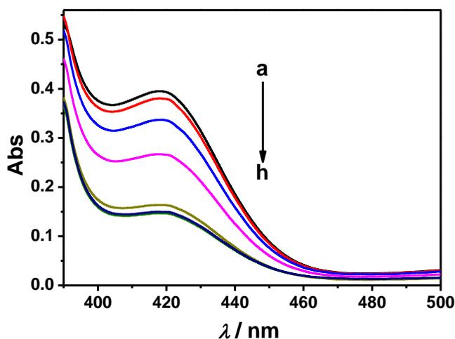
Fig. S8. UV-vis absorption spectra for utilizing  $0.1\ \mu\text{M}$  DNAzyme to analyze different concentrations of  $\text{Pb}^{2+}$ : 0 nM (curve a),  $10^{-9}$  M (curve b),  $10^{-8}$  M (curve c),  $10^{-7}$  M (curve d),  $10^{-6}$  M (curve e),  $10^{-5}$  M (curve f),  $5 \times 10^{-4}$  M (curve g),  $10^{-4}$  M (curve h).
