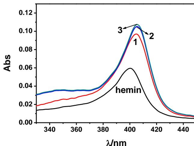
Fig. S4. UV-vis absorption spectra of 1  $\mu\text{M}$  hemin in 20 mM Tris-ClO<sub>4</sub> buffer (pH = 7.4) in the absence and presence of (1) 1  $\mu\text{M}$  Hairpin DNA 1 + 140 mM Na<sup>+</sup>; (2) 10 mM K<sup>+</sup> + (1); (3) 10  $\mu\text{M}$  Pb<sup>2+</sup> + (1), then + 10 mM K<sup>+</sup>.
