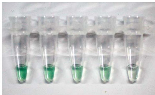
Fig.S5. Colorimetric detection of reaction product of different concentration of target HIV RNA after hemin, ABTS and \text{H}_2\text{O}_2 were added. From left to right: containing 600pM, 60pM, 6pM, 600fM, 0M of HIV RNA, respectively.
