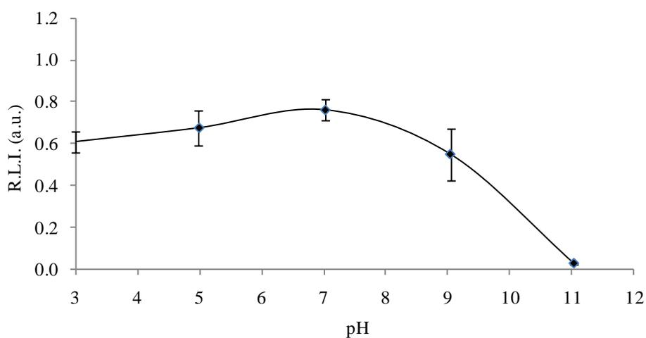
**Fig. S4.** Effect of pH on the complex luminescence intensity in water.  $[\text{Eu}^{3+}] = 5.0 \times 10^{-7} \text{ M}$  and  $[\text{Ligand}] = 2.0 \times 10^{-6} \text{ M}$ .
