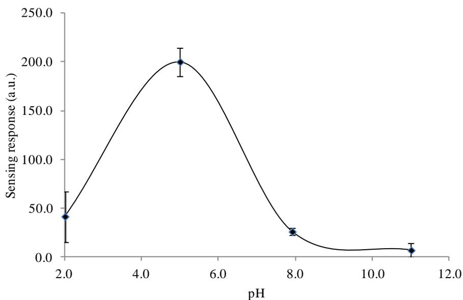
**Fig. S11.** Effect of pH on solid phase. Optimum membrane composition: Nafion:Ligand as 262.3:0.6 mg mL<sup>-1</sup>. [Eu<sup>3+</sup>] = 1.0 x 10<sup>-6</sup> M.  $\lambda_{exc/em}$  = 229.06/616.02 nm, excitation and emission slit widths of 5 nm, 700 V detector voltage,  $t_d$  = 120  $\mu$ s and  $t_g$  = 5 ms.
