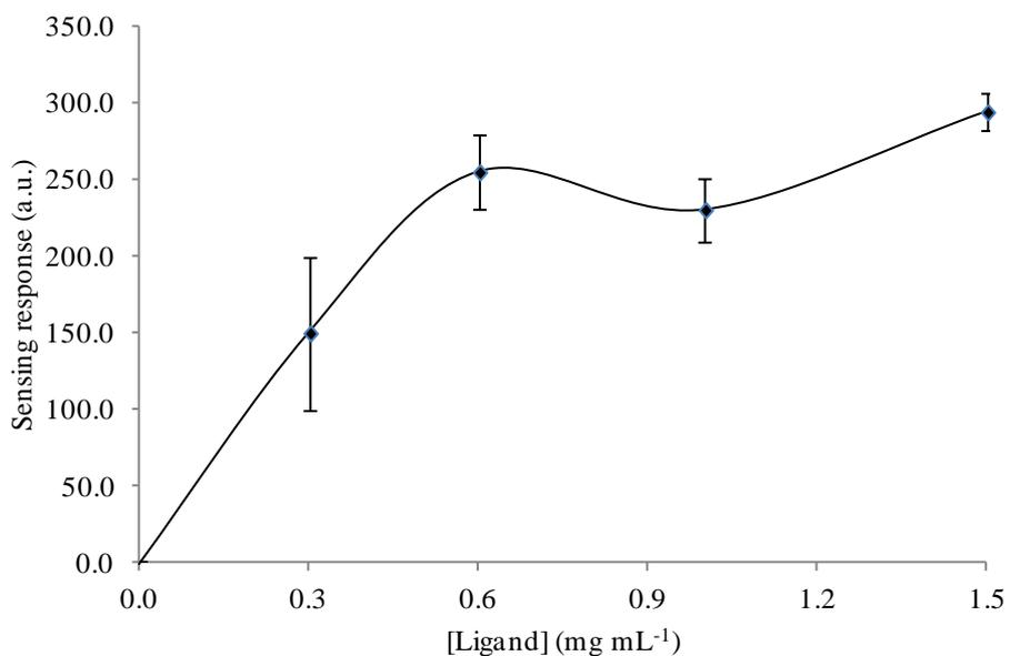
**Fig. S9.** Effect of ligand concentration on the sensing response. Membrane composition: Nafion:Ligand:KTpCIPB as 262.3:0-1.5:0.6 mg mL<sup>-1</sup>. [Eu<sup>3+</sup>] = 1.0 x 10<sup>-6</sup> M.  $\lambda_{exc/em}$  = 229.06/616.02 nm, excitation and emission slit widths of 5 nm, 700 V detector voltage,  $t_d$  = 120  $\mu$ s and  $t_g$  = 5 ms.
