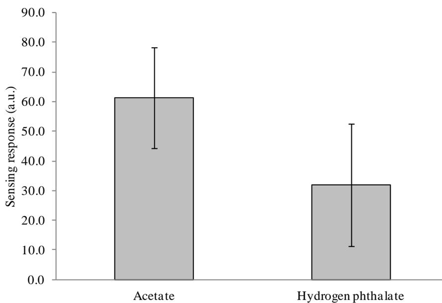
**Fig. S12.** Sensing response of the film in different 75 mM buffer solutions at pH = 5.0. Optimum membrane composition: Nafion:Ligand as 262.3:0.6 mg mL<sup>-1</sup>. [Eu<sup>3+</sup>] = 1.0 x 10<sup>-6</sup> M.  $\lambda_{exc/em}$  = 229.06/616.02 nm, excitation and emission slit widths of 10 nm, 500 V detector voltage,  $t_d$  = 120  $\mu$ s and  $t_g$  = 5 ms.
