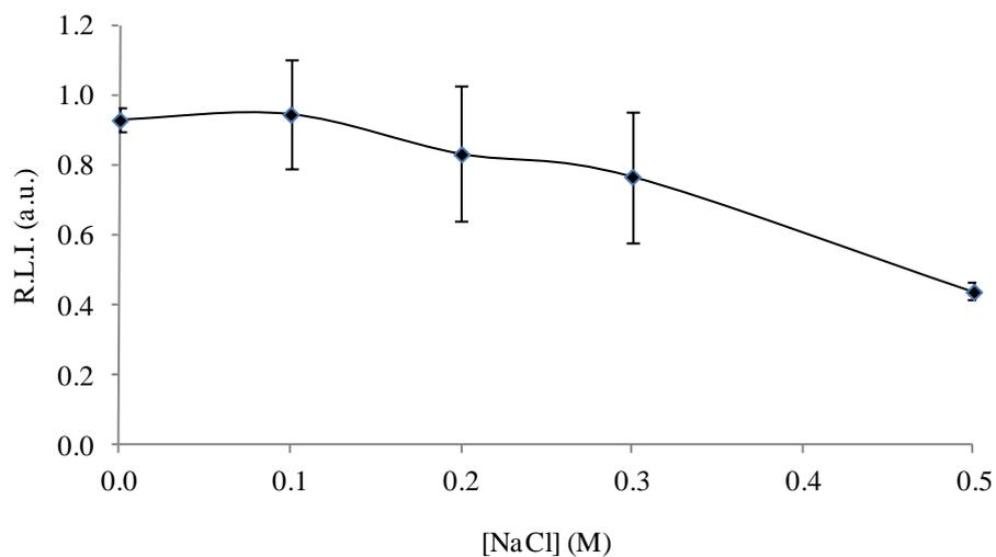
**Fig. S3.** The influence of NaCl concentration on the 1:2 europium(III)-ligand complex luminescence intensity in water.  $[\text{Eu}^{3+}] = 5.0 \times 10^{-7} \text{ M}$  and  $[\text{Ligand}] = 2.0 \times 10^{-6} \text{ M}$ .
