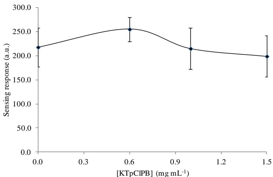
**Fig. S10.** Variation of the sensing response versus ionic additive concentration. Membrane composition: Nafion:Ligand:KTpCIPB as 262.3:0.6:0-1.5 mg mL<sup>-1</sup>. [Eu<sup>3+</sup>] = 1.0 x 10<sup>-6</sup> M.  $\lambda_{exc/em}$  = 229.06/616.02 nm, excitation and emission slit widths of 5 nm, 700 V detector voltage,  $t_d$  = 120  $\mu$ s and  $t_g$  = 5 ms.
