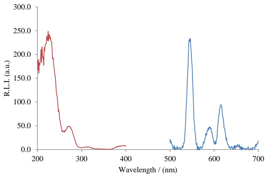
**Fig. S15.** Excitation and emission spectrum of the sensing film in presence of Tb(III) ion.
