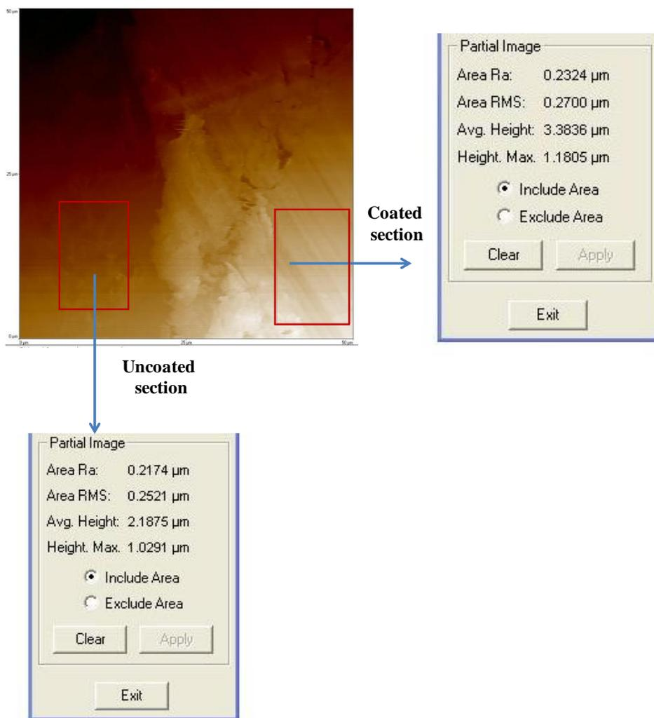
**Fig. S7.** Analysis of roughness and average height of coated and uncoated sections
