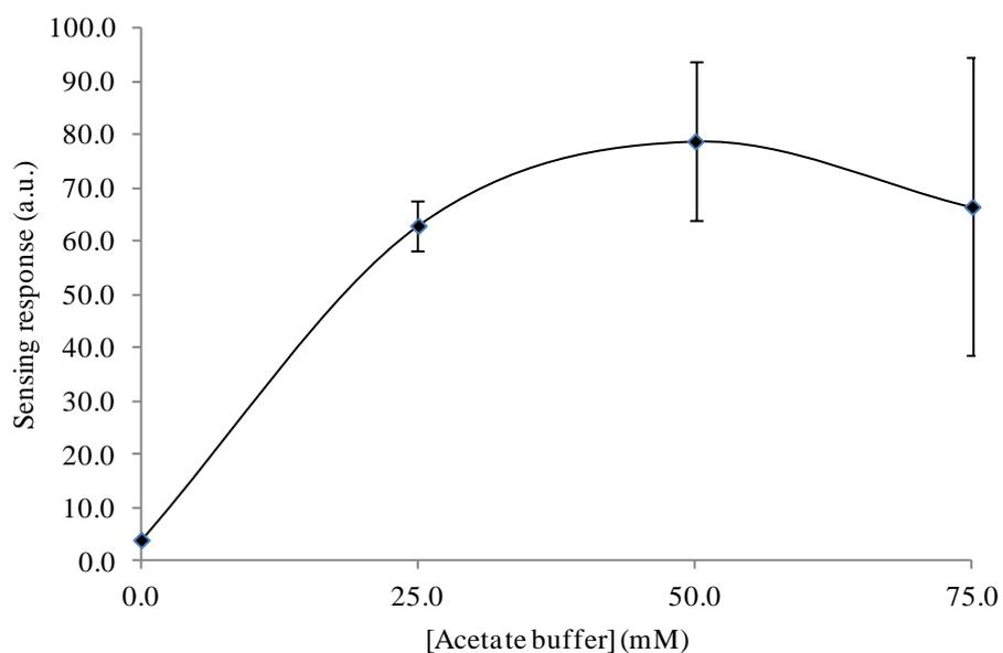
**Fig. S13.** Effect of the ionic strength on the sensing response. Optimum membrane composition: Nafion:Ligand as 262.3:0.6 mg mL<sup>-1</sup>. [Eu<sup>3+</sup>] = 1.0 x 10<sup>-6</sup> M, pH = 5.0.  $\lambda_{\text{exc/em}}$  = 229.06/616.02 nm, excitation and emission slit widths of 10 nm, 500 V detector voltage,  $t_d$  = 120  $\mu$ s and  $t_g$  = 5 ms.
