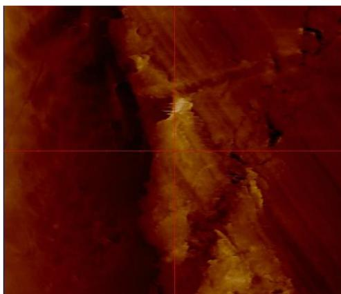
**Fig. S6.** 2D Image of AFM in which is possible to distinguish the scanning direction (red line) and the concentric lines which appear in the coated section (resolution 1024 lines, size 50 x 50  $\mu\text{m}$ ).
