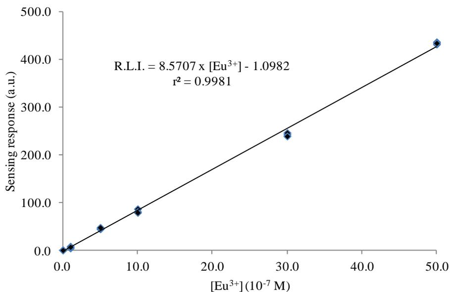
**Fig. S14.** Calibration graph of the europium(III) membrane sensors. Optimum membrane composition: Nafion:Ligand as 262.3:0.6 mg mL<sup>-1</sup>. [Blank] = 25 mM acetate buffer at pH 5.0; [Eu<sup>3+</sup>] = 1.0 x 10<sup>-7</sup> - 5.0 x 10<sup>-6</sup> M in 25 mM acetate buffer solution at pH 5.0.  $\lambda_{\text{exc/em}}$  = 229.06/616.02 nm, excitation and emission slit widths of 10 nm, 500 V detector voltage,  $t_d$  = 120  $\mu$ s and  $t_g$  = 5 ms.
