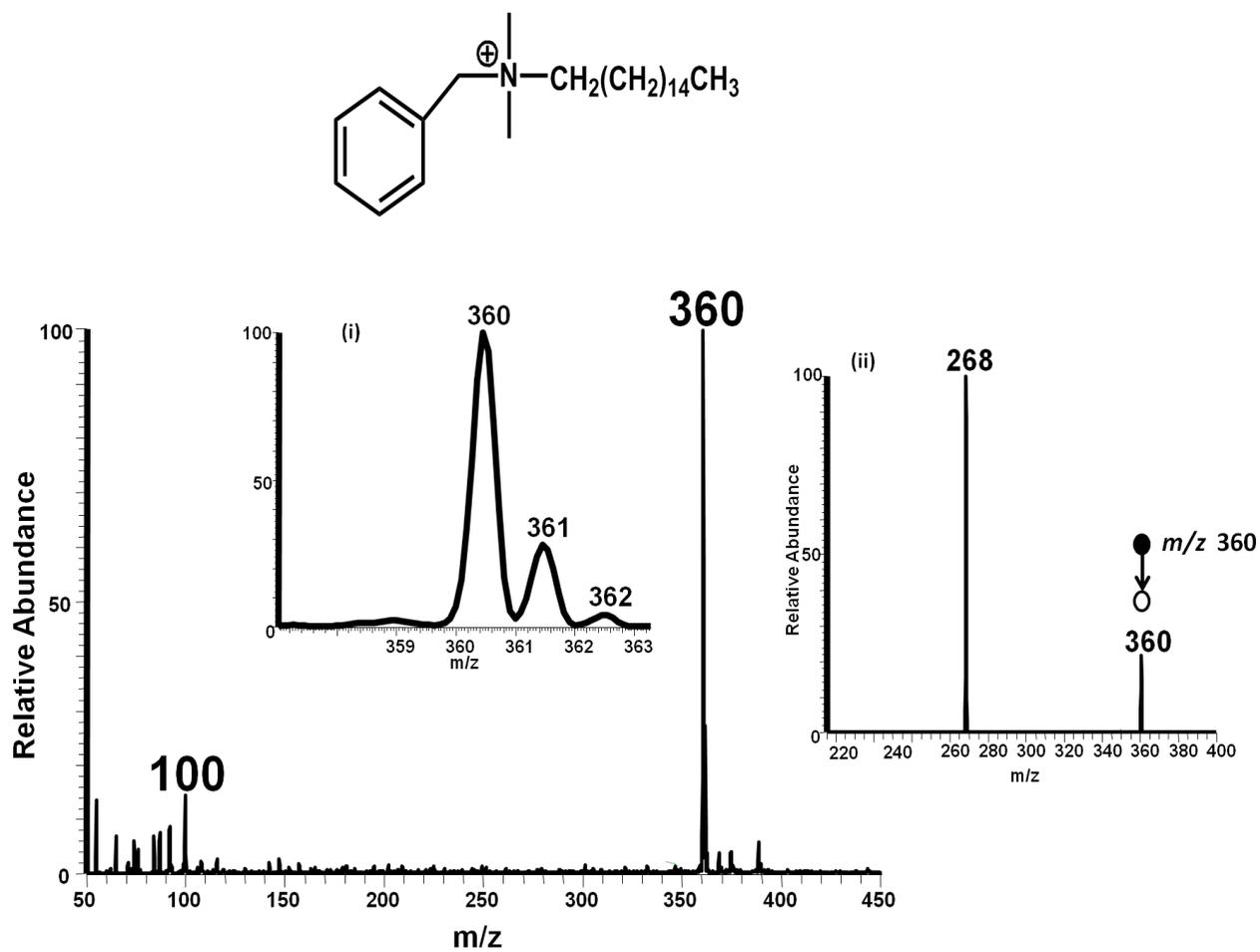
**Figure S6.** Positive ion PS-MS mass spectrum of benylhexadecyldimethylammonium chloride. Insert (i) shows the Isotopic distribution of the analyte ion, (ii) Tandem mass spectrometry (MS/MS) of the benylhexadecyldimethylammonium cation at  $m/z$  360 gives a major fragment ion at  $m/z$  268 with a loss of alkene  $-[92]$  that confirms the structure
