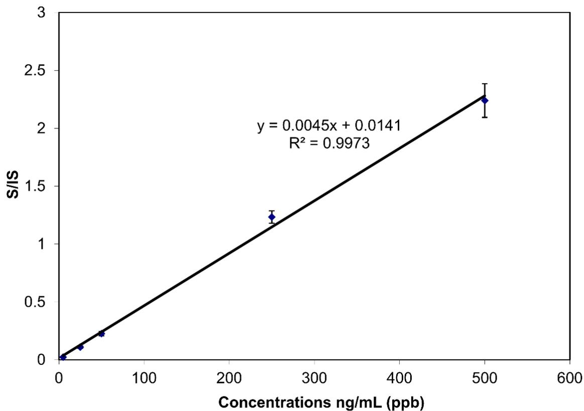
**Fig S1.** Calibration curve for the quantitative analysis of ammonium salts in oil matrix using a commercial ion trap mass spectrometer
