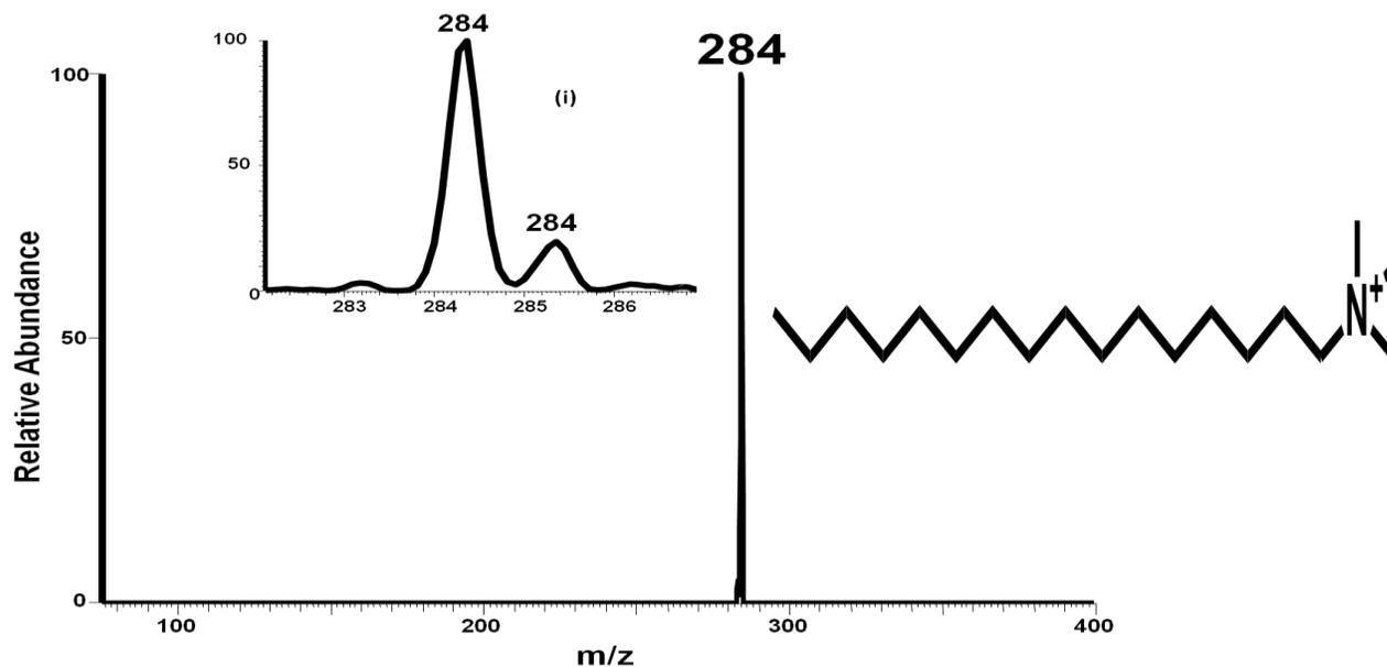
**Figure S3.** Positive PS-MS mass spectrum of hexadecyltrimethylammonium bromide. Insert (i) shows the isotopic distribution of the analyte, tandem mass spectrometry (MS/MS) of the hexadecyltrimethylammonium cation at  $m/z$  284.0 was not returning good signal since the expected major fragment is below the low mass cut off the instrument.
