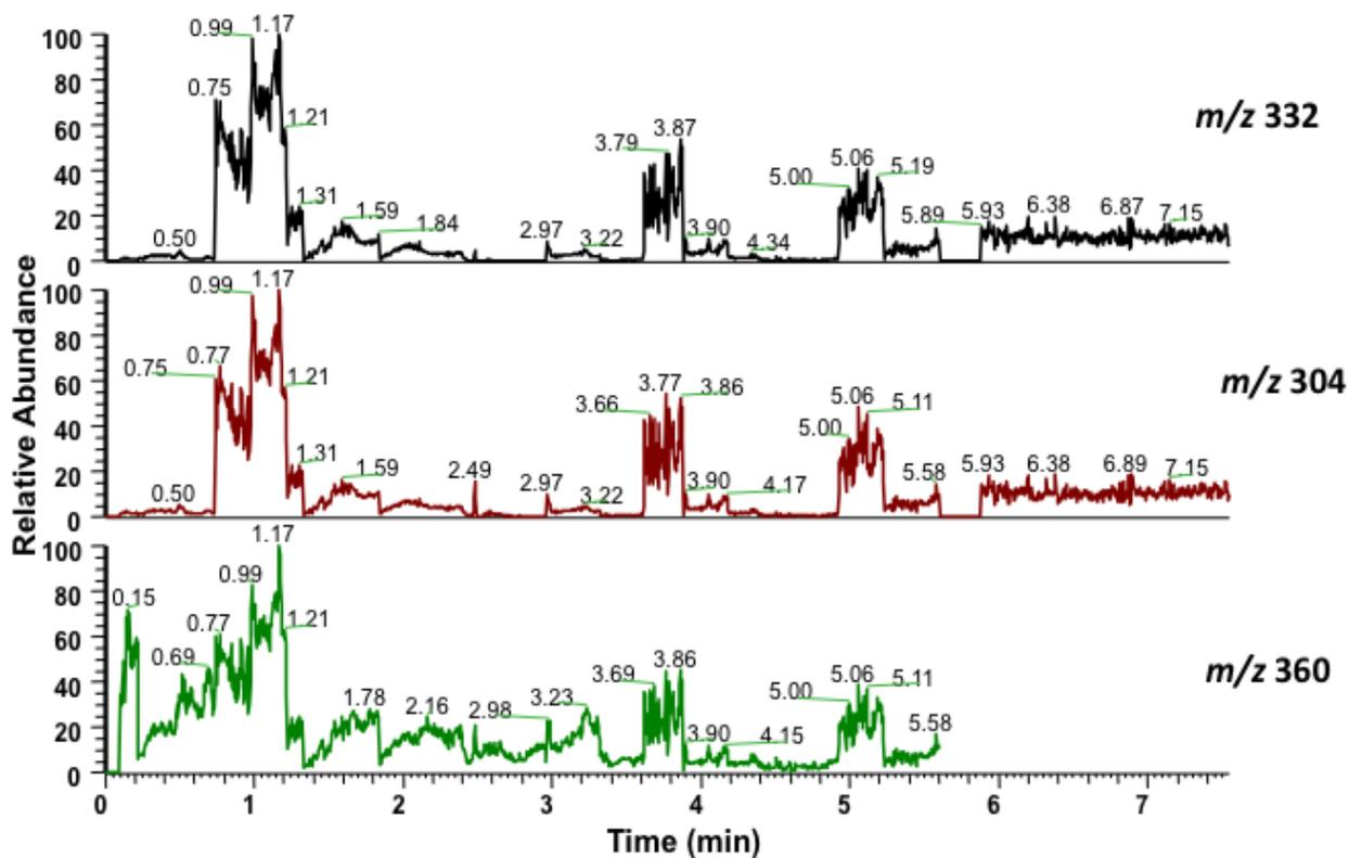
**Figure S9.** Ion chromatograms for the for alkyl dimethylbenzyl ammonium chloride  $[\text{C}_6\text{H}_5\text{CH}_2\text{N}(\text{CH}_3)_2\text{R}]\text{Cl}$  where R is predominantly  $n\text{-C}_{12}\text{H}_{25}$ ; data for the homologs  $\text{C}_{14}$  ( $m/z$ ) 332,  $\text{C}_{12}$  ( $m/z$ ) 304, and  $\text{C}_{16}$  ( $m/z$ ) 360 are shown.
