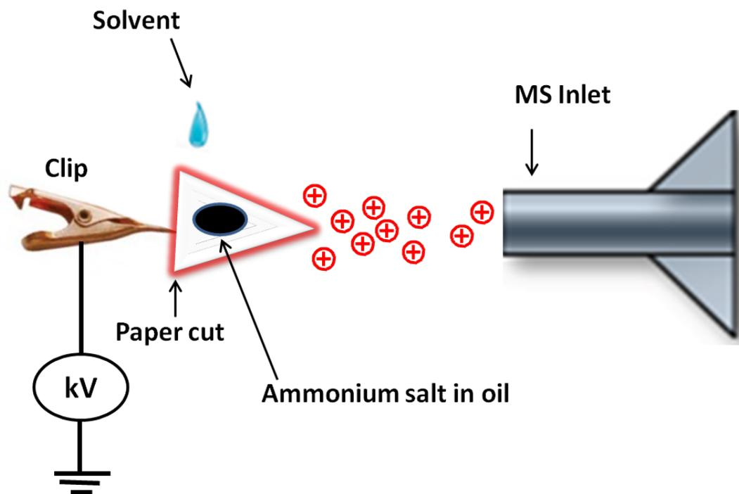
**Figure S2.** Paper spray ionization mass spectrometry for *in situ* analysis of corrosion inhibitors using a commercial benchtop mass spectrometer
