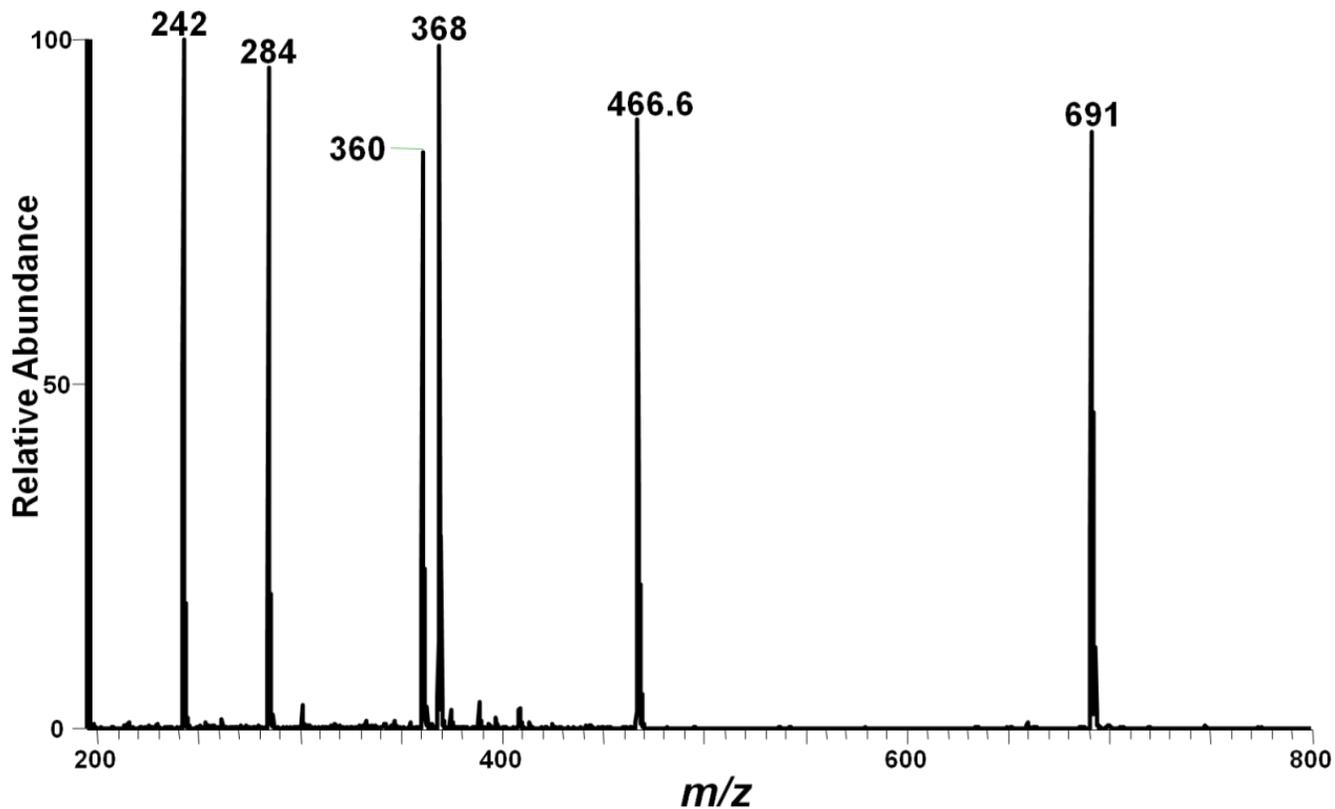
**Figure S7.** Positive ion mode paper spray mass spectrum for artificial mixtures of model compounds analyzed using a benchtop instrument. Tetrabutylammonium bromide was observed at  $m/z$  242.0, hexadecyltrimethylammonium bromide at  $m/z$  284.0, benzylhexadecyldimethylammonium chloride at  $m/z$  360.0, tetraoctylammonium bromide at  $m/z$  466.6 and tetradodecylammonium bromide at  $m/z$  691.0.
