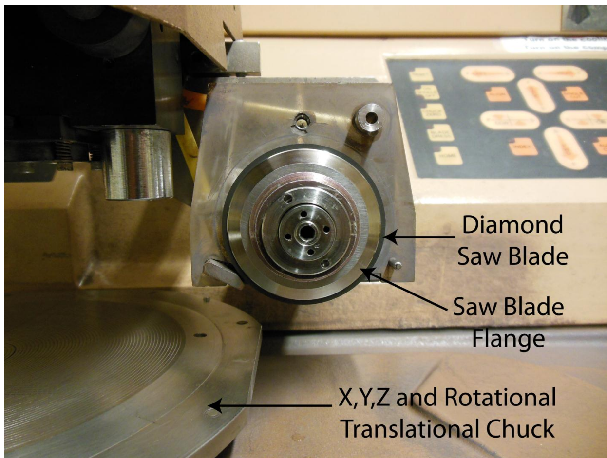
Fig. S2 Close-up of the micro-dicing saw. The diamond saw blade is held by compression in the saw blade flange. When cuts are made the blade assembly remains fixed while the x, y, z, and rotational translation chuck performs the necessary movements to accomplish the desired cuts.
