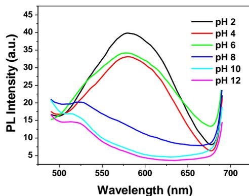
**Figure S5.** PL spectra of bare LPSiNPs incubated in aqueous solution with different pH values, with an excitation of 365 nm.
