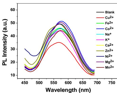
**Figure S7.** PL spectra of bare LPSiNPs incubated in aqueous solution (pH 7.4) containing different metal ions, with an excitation of 365 nm.
