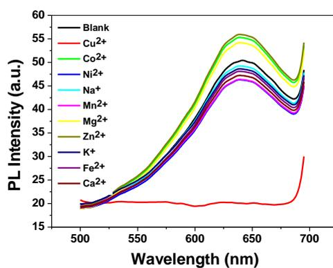
**Figure S6.** PL spectra of UA-LPSiNPs incubated in aqueous solution (pH 7.4) containing different metal ions (20  $\mu\text{mol/L}$ ), with an excitation of 365 nm.
