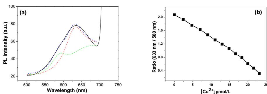
**Figure S9.** (a) multi-gaussian fitting of PL spectra of UA-LPSiNPs, (b) the relationship between the ratio of 633 nm/580 nm and the concentration of adding Cu<sup>2+</sup>.
