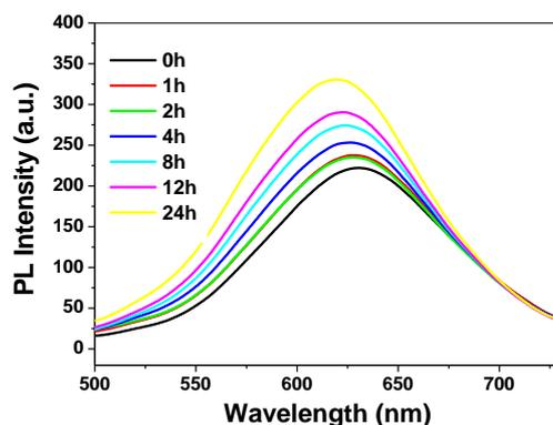
**Figure S1.** PL spectra of UA-LPSiNPs incubated in PBS solution (pH 7.4) at 37 °C for different hours, with an excitation of 380 nm.
