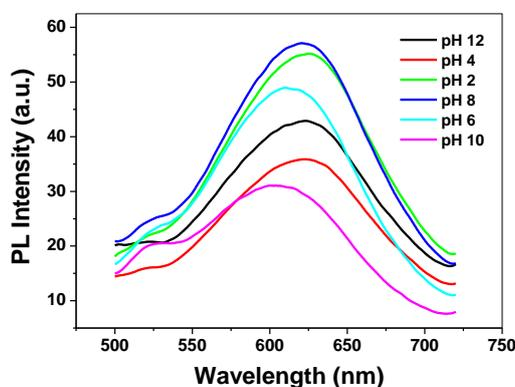
**Figure S3.** PL spectra of UA-LPSiNPs incubated in aqueous solution with different pH values, with an excitation of 380 nm.
