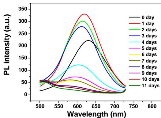
**Figure S2.** PL spectra of UA-LPSiNPs incubated in PBS solution (pH 7.4) at 37 °C for different days, with an excitation of 380 nm.
