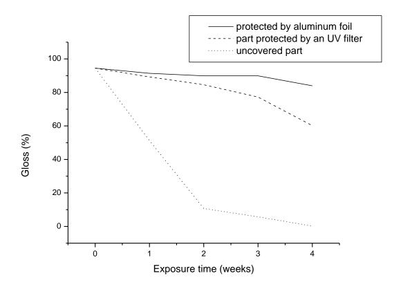
**Supplementary Figure 1s:** gloss measurements during the artificial ageing of sample boards (Glossmeter Zehntner ZLR 1050 M with a spectral relection angle of 60°)
