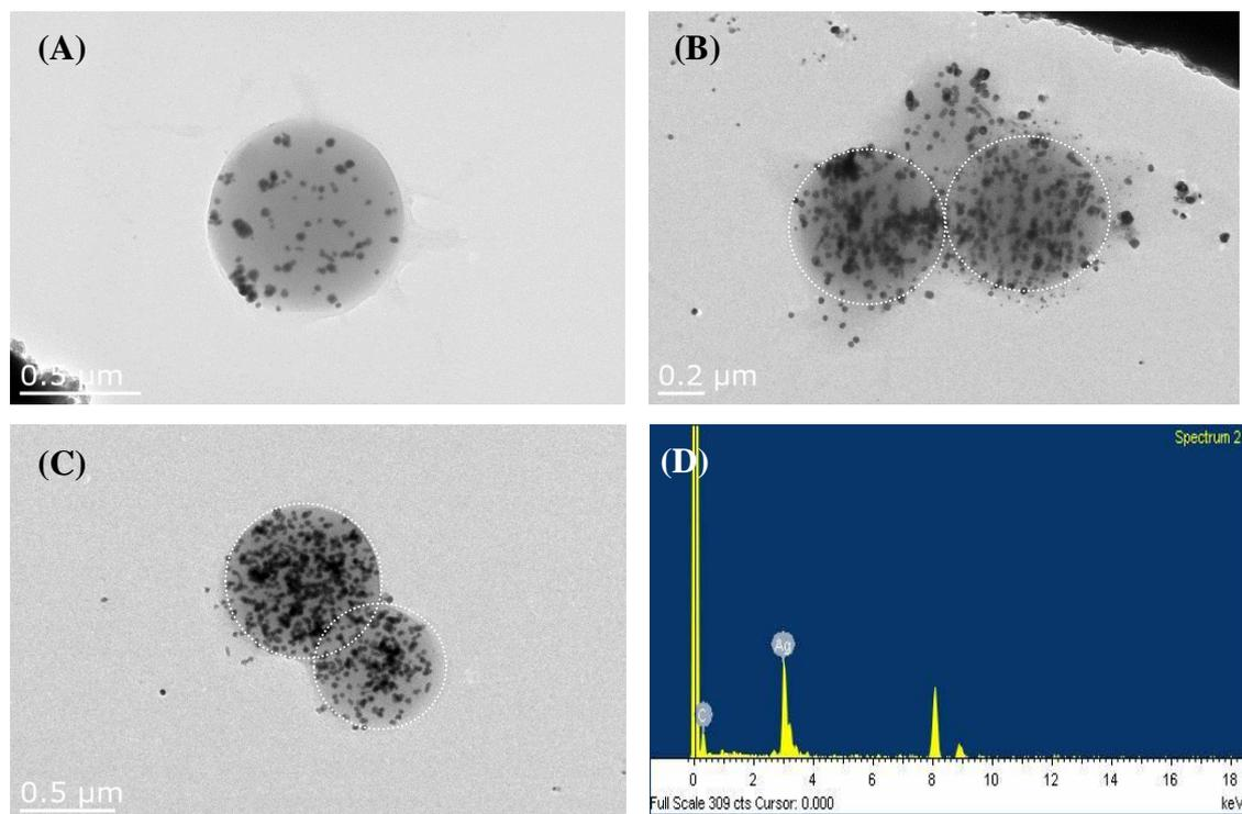
**Figure S3.** TEM images of Ag NC-embedded polymer NPs at Ag NC concentration of (A) 0.2 w/v%, (B) 0.6 w/v% and (C) 0.8 w/v% in the jetting solution. (D) Energy dispersive x-ray spectrum (EDS) of Ag NCs, indicating the presence of Ag.
