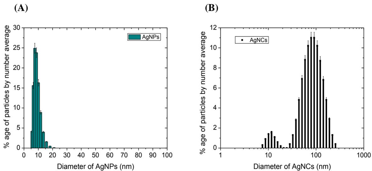
**Figure S1.** Diameter and size distribution of (A) discrete Ag NPs and (B) Ag NCs, determined by dynamic light scattering (DLS).
