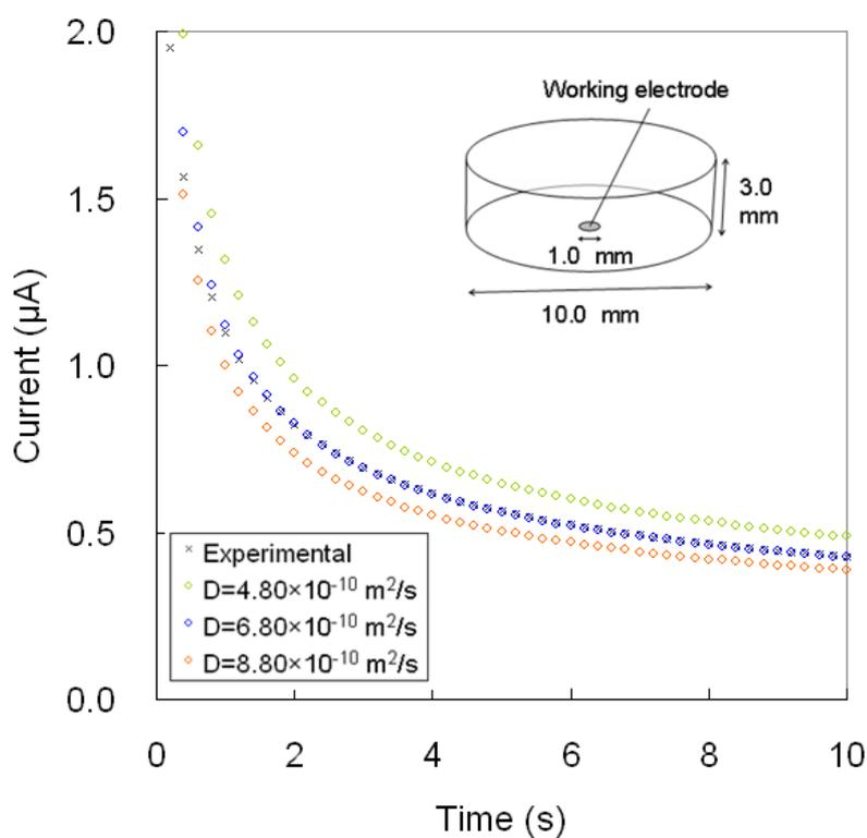
Figure S2. Curve fitting of the experimental data to the COMSOL simulation to determine the diffusion coefficient of pAP.
