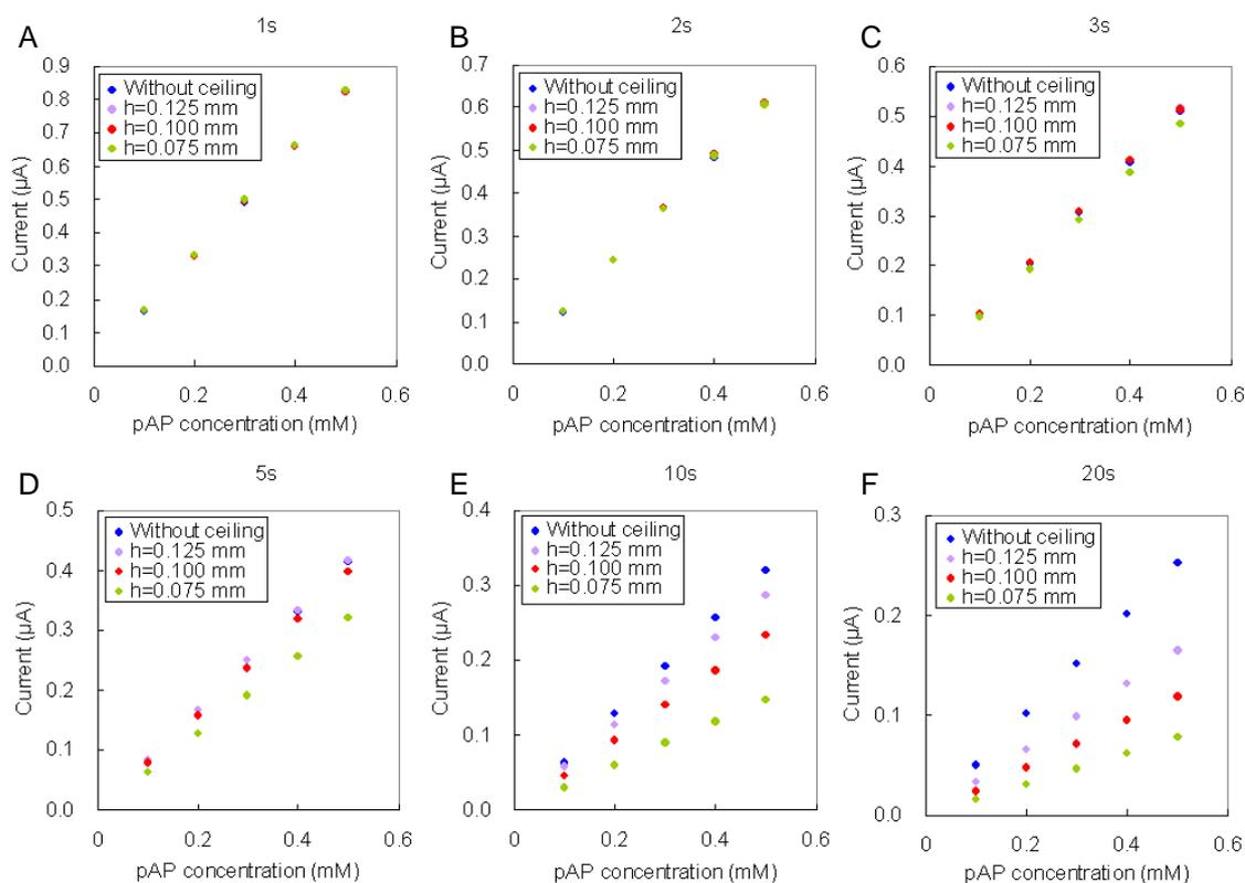
Figure S3. Simulated calibration lines for the chip sensor with various heights of the reaction chamber ( $h = 3.0$  mm (free diffusion without ceiling), 0.125 mm, 0.100 mm and 0.075 mm in Fig. 7A). Currents at 1s (A), 2 s (B), 3 s (C), 4 s (D), 5 s (E), and 6 s (F) after the potential step serving as the signal.
