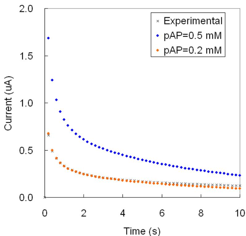
Figure S4. Comparison of experimental data and simulated curve for amperometry with the chip sensor.
