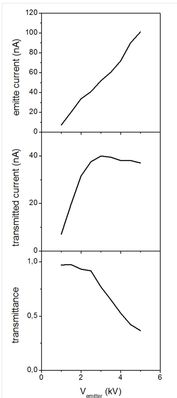
**Figure S-2:** emission and transmission characteristics showing high transmitted current in vacuum for a  $10^{-4}$  M solution as function of the voltage applied to the emitter. Depending on the emitter characteristics, the current transmitted to vacuum may vary. The data presented here are representative of the highest current recorded in vacuum for the funnel shaped 1 mm diameter capillary.
