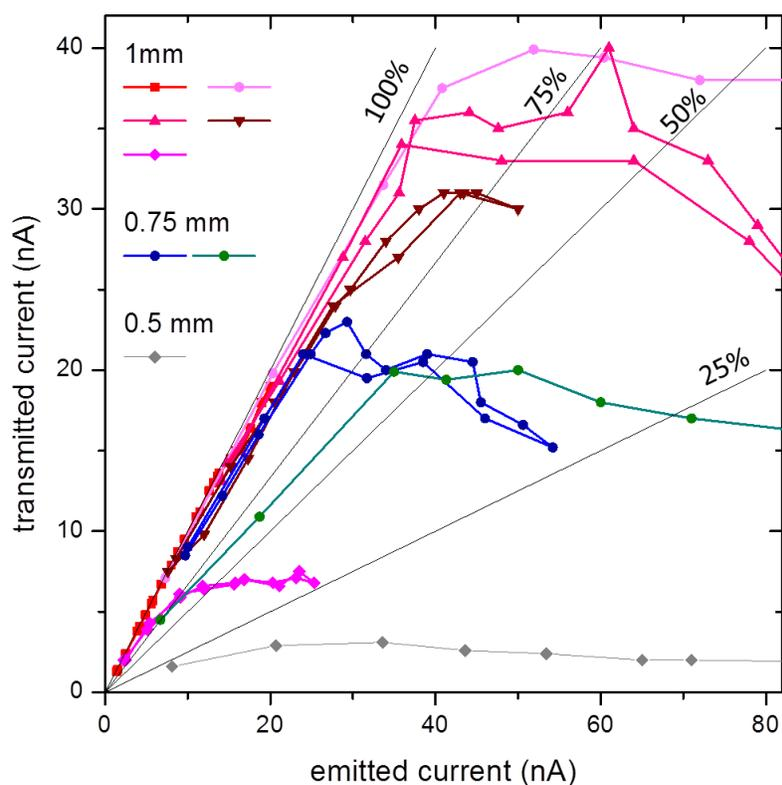
**Figure S-9:** Transmitted current as a function of emitted current at  $V_{ES} = 2.5$  kV for the 1 mm funnel capillary. The emitter was placed at  $z = -6.5$  mm,  $r = 0$  mm and fed with the  $10^{-4}$  M RhoB solution. For comparison, corresponding data are given for the same funnel inlet attached to 0.75 mm and 0.5 mm capillaries.
