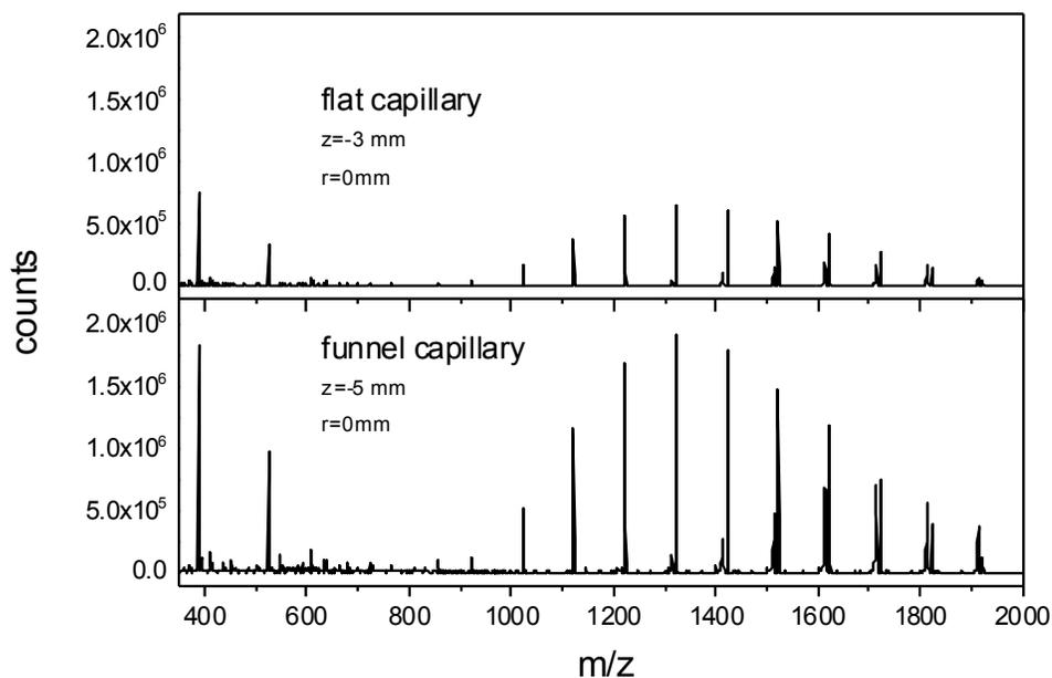
**Figure S-7:** High resolution mass spectra of the positive ion mode calibration solution recorded with an Orbitrap XL ETD mass spectrometer for the flat and the funnel capillaries.
