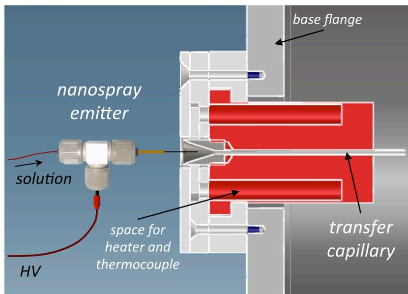
**Figure S-1:** Cross section of the vacuum interface. The length of the capillary including the funnel is 7 cm.
