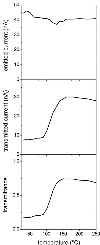
**Figure S-8:** Temperature dependence of the transmission of the funnel interface of a 1mm capillary.  $V_{ES}=2.5\text{kV}$ ,  $\text{RhoB}$   $c=10^{-4}\text{ M}$ ,  $z=-6.5\text{mm}$ .
