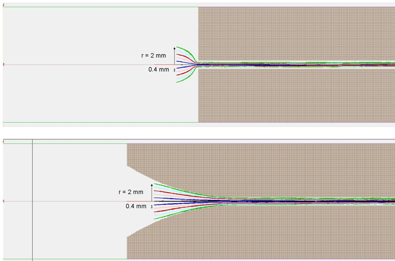
**Figure S-6:** trajectories of 10 ions starting 2.5 mm beyond the ion emitter at various radial positions between  $r = 0$  mm and  $r = 2$  mm.
