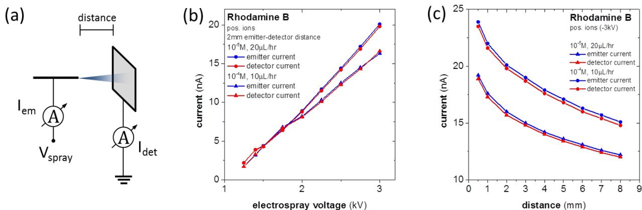
**Figure S-4:** a) Layout of the reference experiment. b) Absolute value of emitted and collected current as function of the electro spray voltage and c) as a function of the distance.
