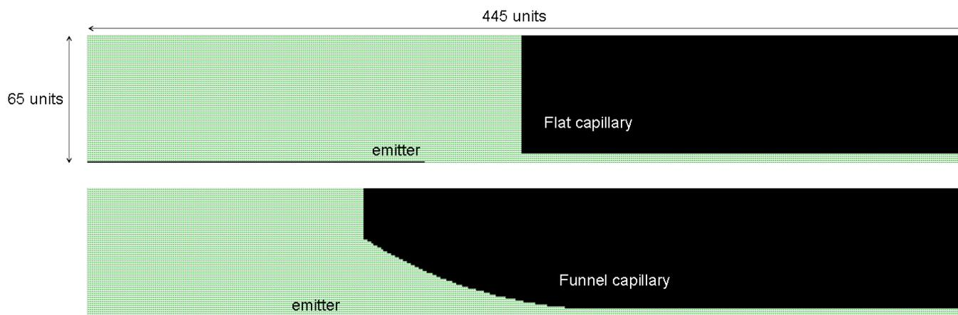
**Figure S-5:** potential arrays used for the flat and the funnel capillary for the simulations with SIMION.
