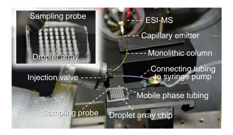
Figure S1. Setup of the droplet array-LC/MS system.
