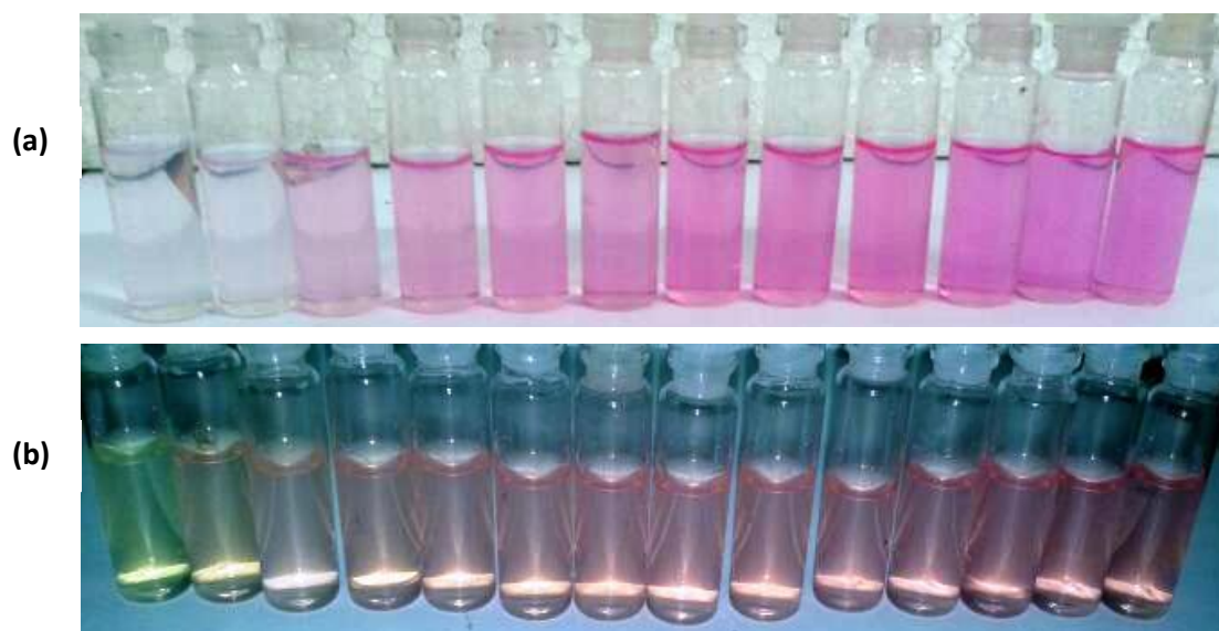
Fig. S35 Visual color change of (a) L^1 and (b) L^2 with increase of concentration of Hg^{2+} ions added (0-30 \mu M ) in HEPES buffer (1 mM, pH 7.4; DMSO/water: 1/9, v/v) at 25 °C.
