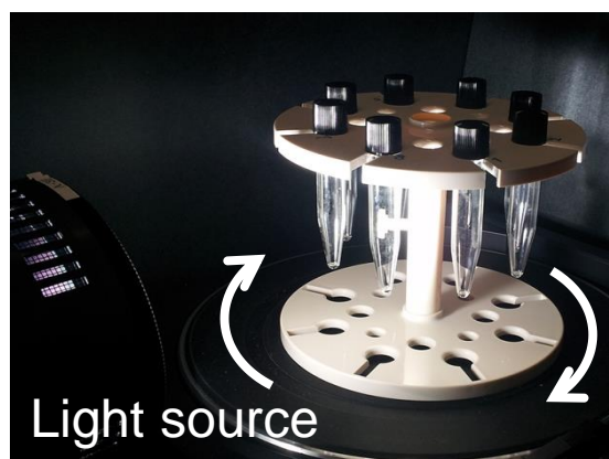
Fig. S2 Merry-go-round reaction system for photocatalytic reactions. Eight test tubes can be set up at the same time.
