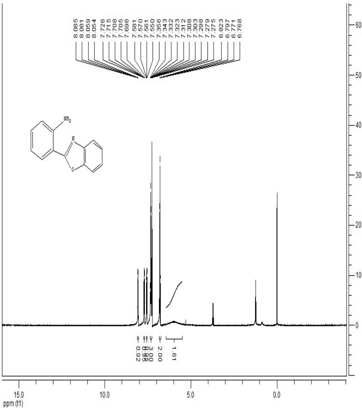
**Figure S-13.** The  $^1\text{H}$  NMR spectra of 1 in  $\text{CDCl}_3$
