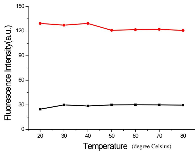
**Figure S-5.** The fluorescence spectra of compound NBPA (10  $\mu\text{M}$ ) before (black line) and after (red line) addition of 1.0 equiv of  $\text{Zn}^{2+}$  at different temperatures in  $\text{CH}_3\text{CN}/\text{H}_2\text{O}$ (1:1, v/v); entrance slit, 2.5 nm; exit slit, 2.5 nm; t, 10 min.
