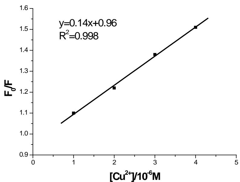
**Figure S-6.** Stern-Volmer plot to estimate fluorescence quenching for complex NBPA- $\text{Zn}^{2+}$  in the presence of  $\text{Cu}^{2+}$ .
