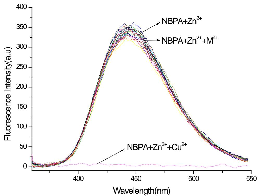
**Figure S-8.** Fluorescence spectra of NBPA-Zn<sup>2+</sup> and the addition of various ions to NBPA-Zn<sup>2+</sup> in CH<sub>3</sub>CN-buffer solution (1:1, v/v); NBPA-Zn<sup>2+</sup>, 1.0 × 10<sup>-5</sup> M; metal ions, 1.0 × 10<sup>-5</sup> M; Buffer solution (HAc-NaAc), 0.10 M; entrance slit, 2.5 nm; exit slit, 5 nm; t, 10 min.
