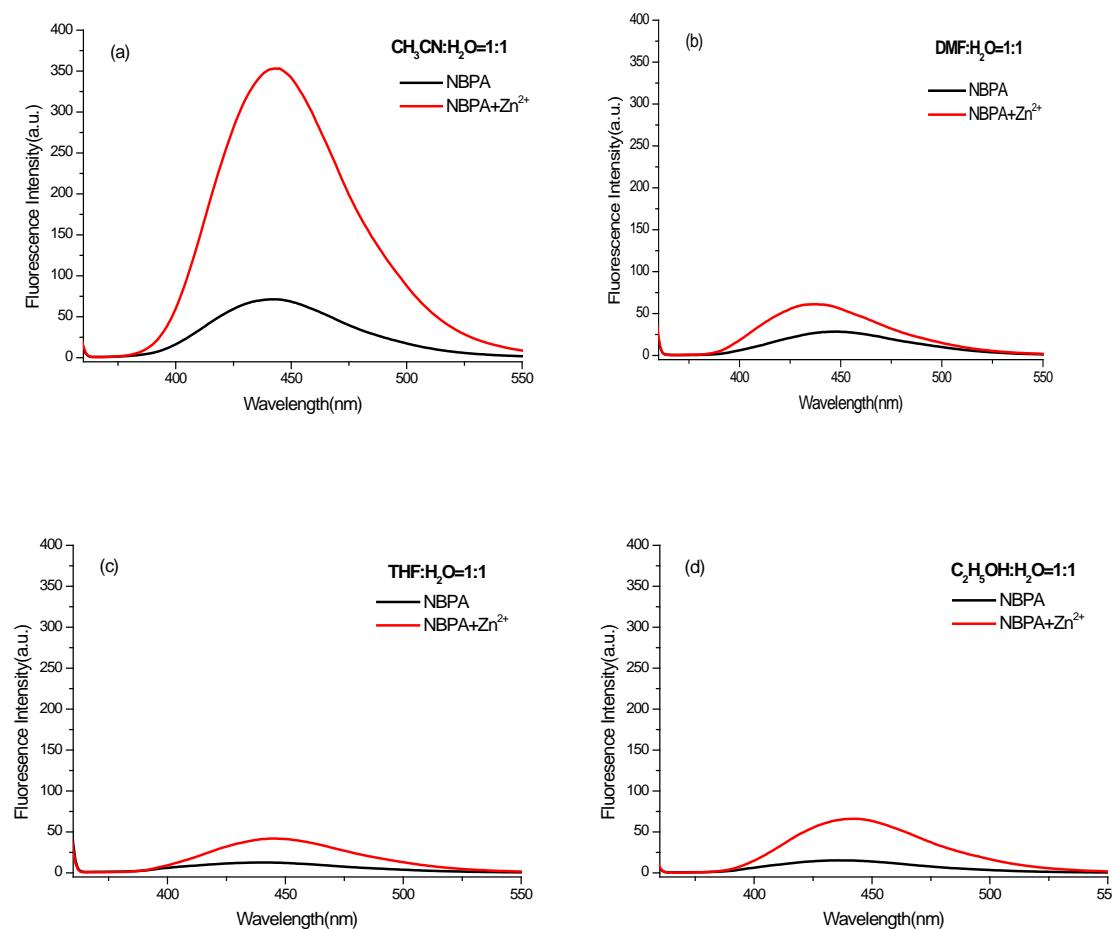
**Figure S-3.** The fluorescence spectra of compound NBPA (10  $\mu\text{M}$ ) before (black line) and after (red line) addition of 1.0 equiv of  $\text{Zn}^{2+}$  in different solvent / $\text{H}_2\text{O}$ (1:1, v/v). a) acetonitrile, b)DMF, c) THF, d) ethanol; entrance slit, 2.5 nm; exit slit, 5 nm; t, 10 min.
