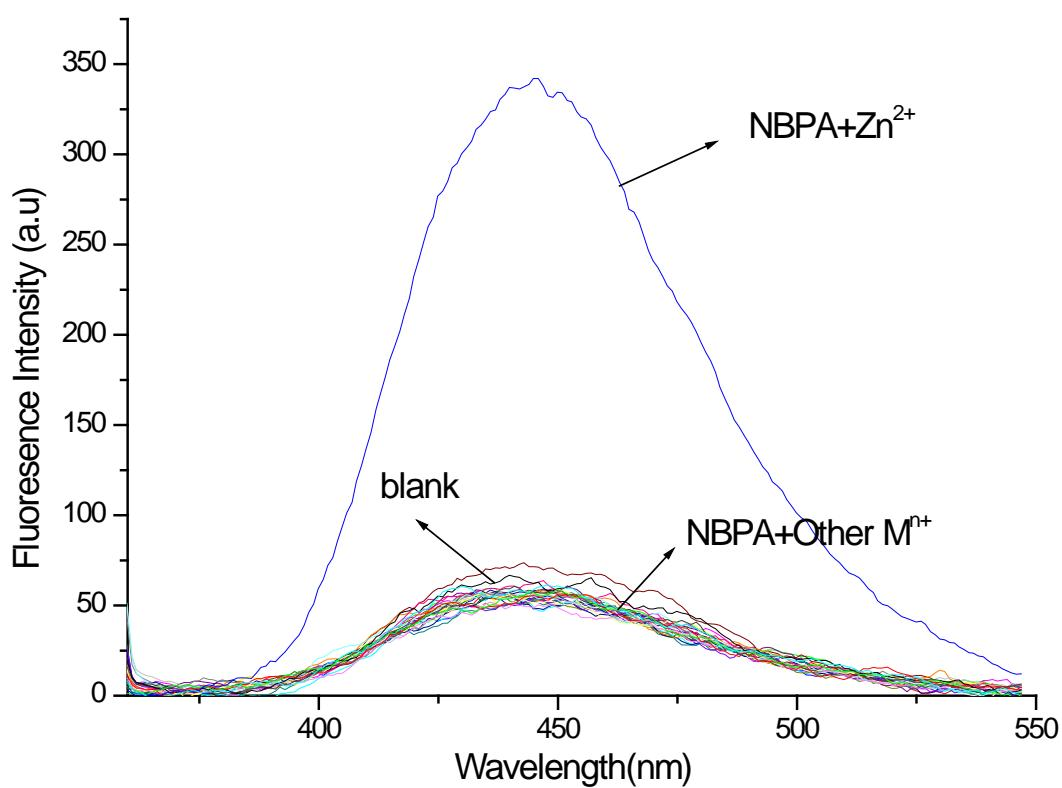
**Figure S-7.** Fluorescence spectra of NBPA and the addition of various ions to NBPA in CH<sub>3</sub>CN- buffer solution (1:1, v/v); NBPA, 1.0 × 10<sup>-3</sup> M; metal ions, 1.0 × 10<sup>-5</sup> M; Buffer solution (HAc-NaAc), 0.10 M; entrance slit, 2.5 nm; exit slit, 5 nm; t, 10 min.
