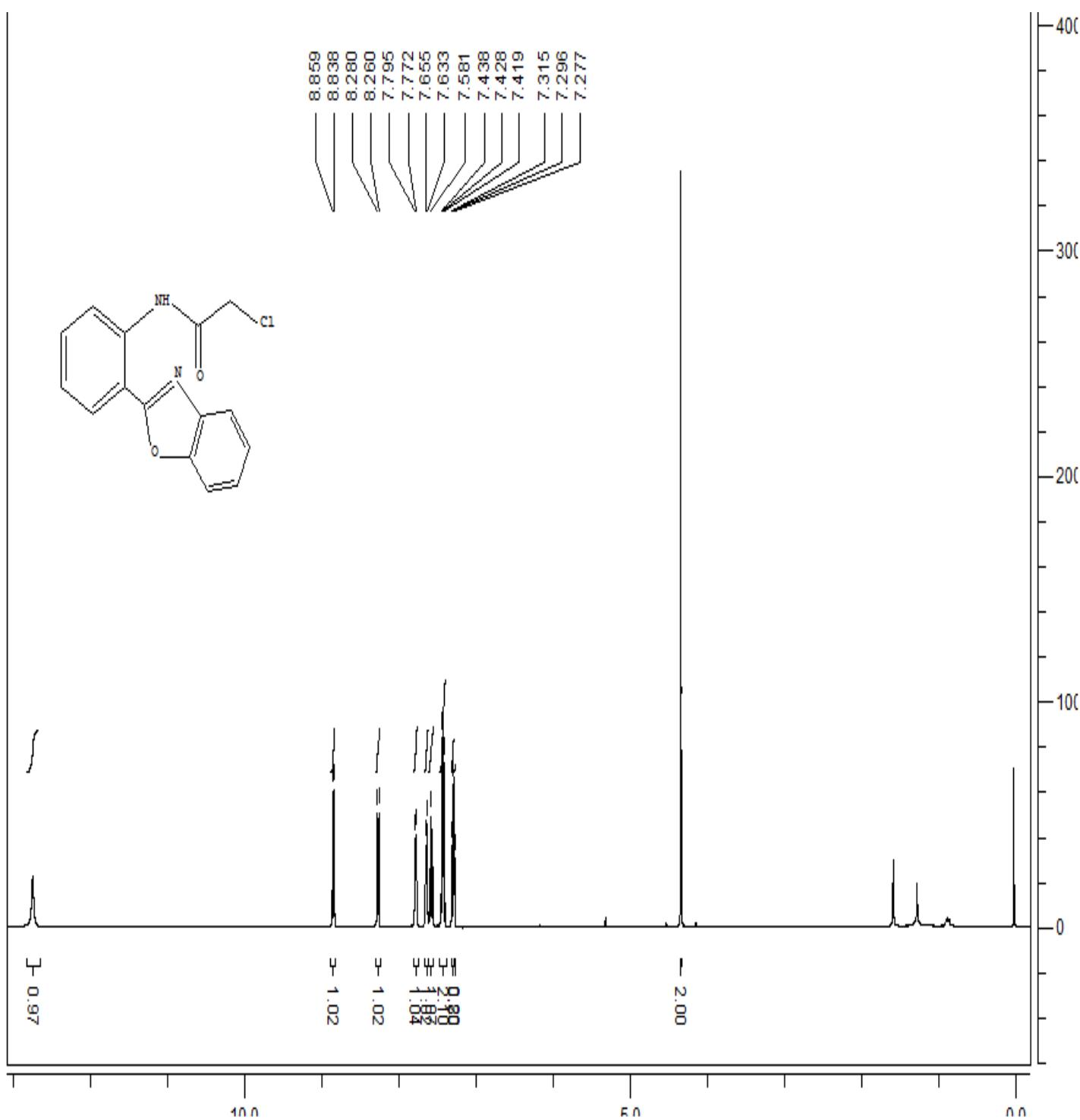
Figure S-14. The <sup>1</sup>H NMR spectra of 2 in CDCl<sub>3</sub>
