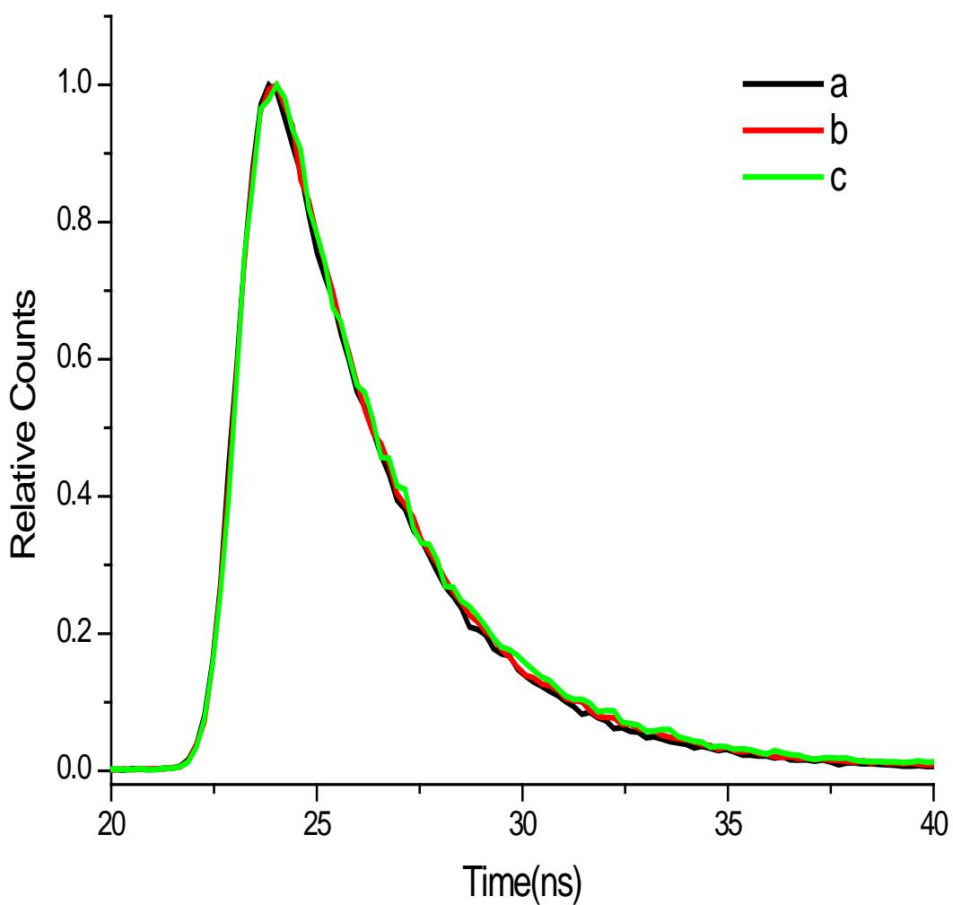
**Figure S-9.** Fluorescence decay curves for NBPA in presence of (a)  $Zn^{2+}$  (b)  $Cu^{2+}$  and (c)  $Zn^{2+}/Cu^{2+}$
