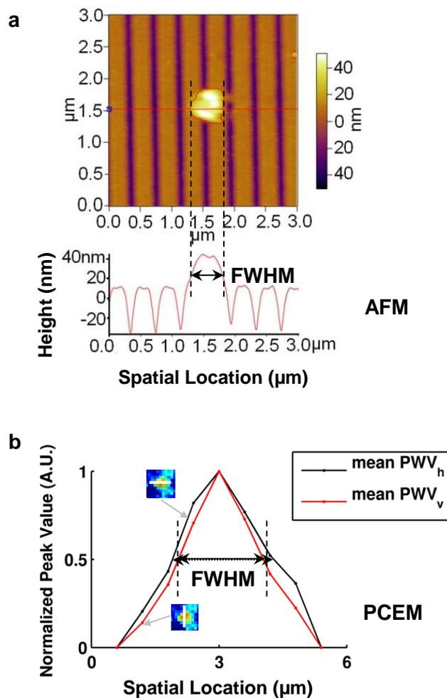
**Supplementary Figure 1. Comparison of FWHM of tDPN nano-dots on the PC surface measured by AFM and PCEM.** (a) tDPN nano-dots measured by AFM, indicating a FWHM (mean) of 540 nm. (b) tDPN nano-dots measured by PCEM, indicating a FWHM (mean) of 1.20 μm in horizontal direction and 1.13 μm in vertical direction (measured from PWV image).
