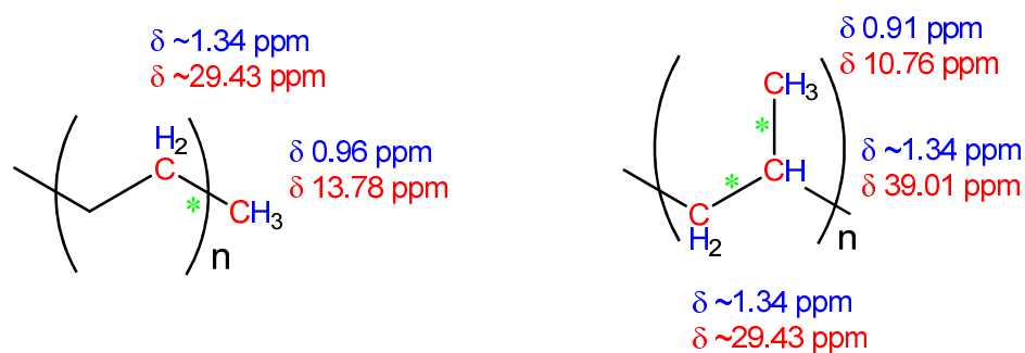
Figure SI7. NMR peak assignment for a sample of film used for LD measurements. Green stars mark the observed crosspeaks in the HMBC spectrum. (left) Polyethylene chain, (right) polypropylene chain.
