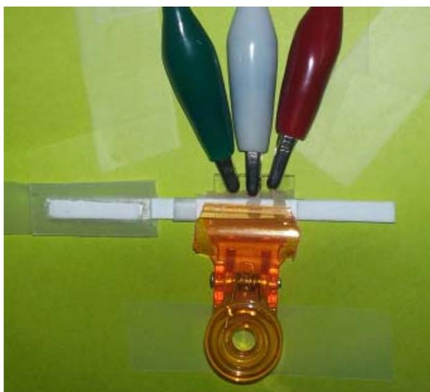
**Fig. S5** Photograph of an electrochemical lateral-flow immunostrip.
