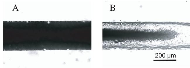
**Fig. S1.** Pictures of PPMs synthesized in a grafted microchannel with PEG diacrylate (A) and in an ungrafted one (B).
